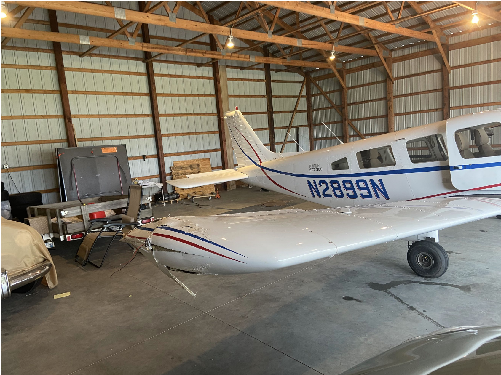
Photo 1 – Right wing damage
