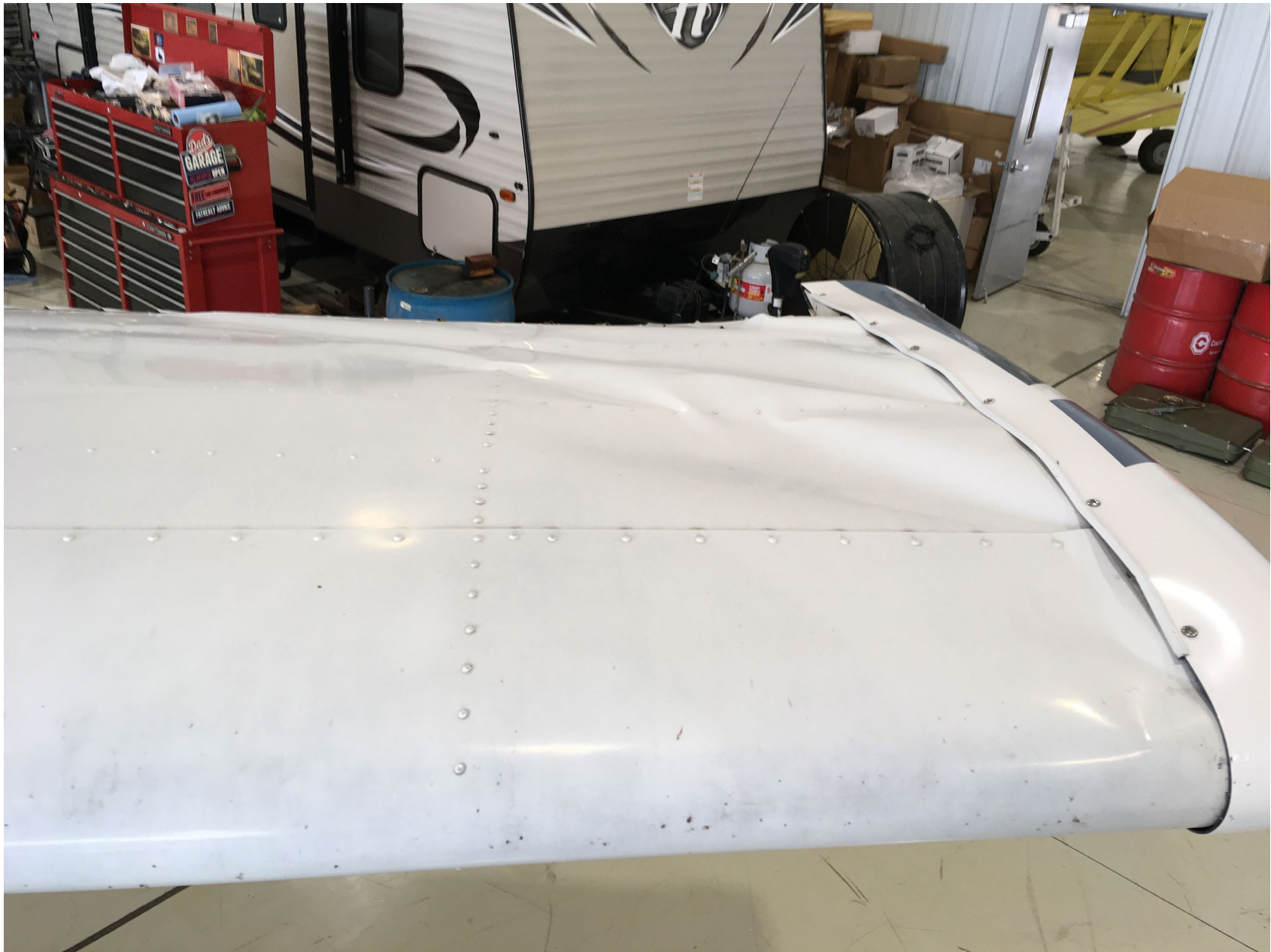
Photo 2 – Left Wing Tip Damage – Courtesy of FAA
