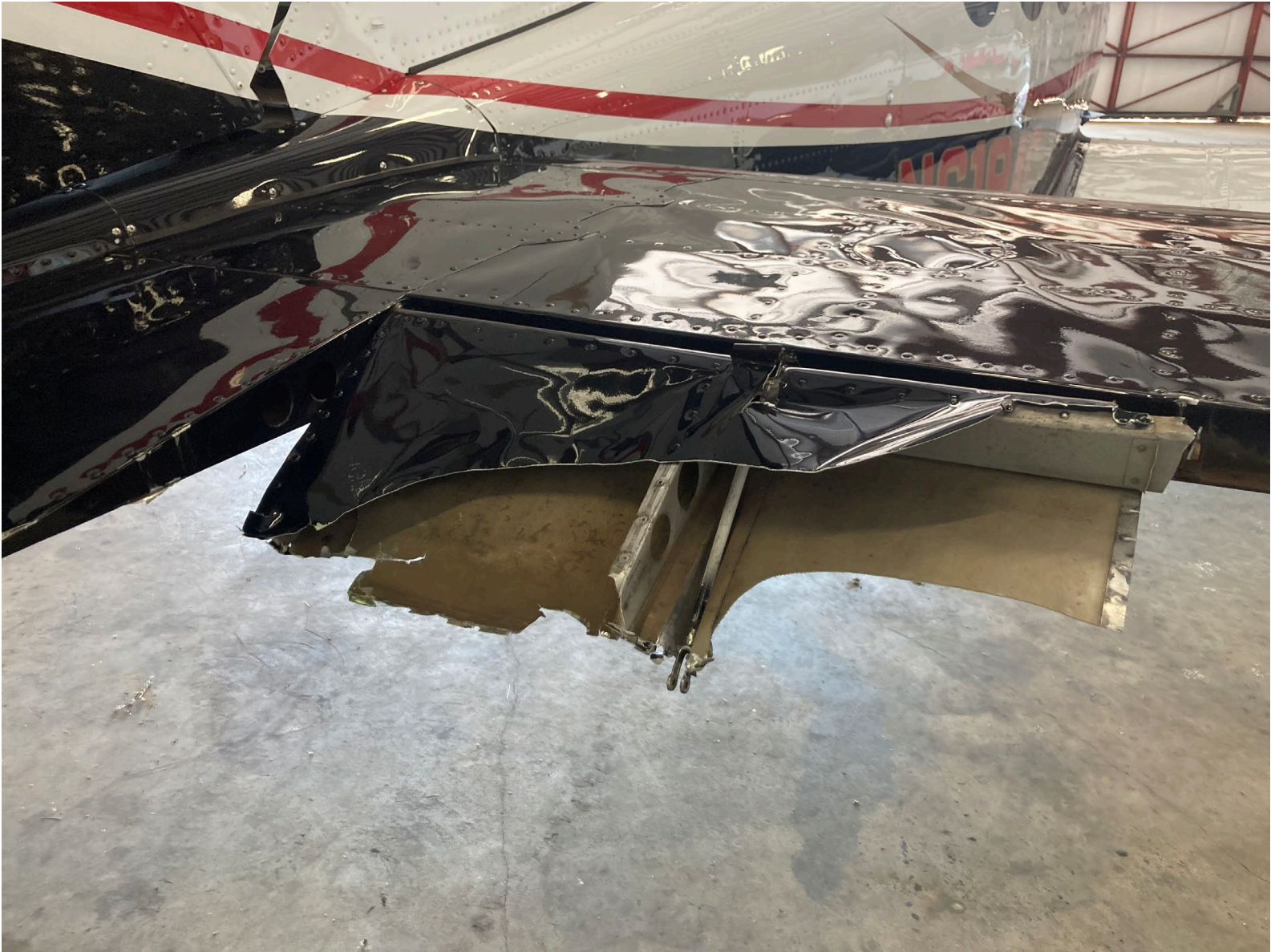
Photograph 3 - Partially separated elevator (Courtesy of FAA)
