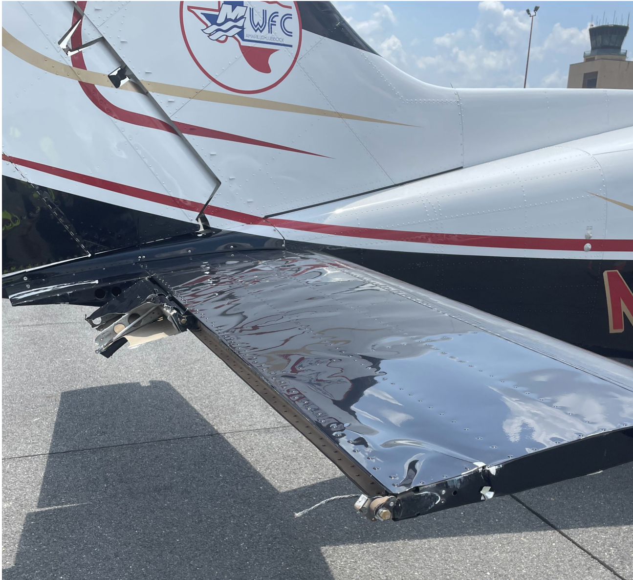
Photograph 1 - Partially separated elevator (Courtesy of FAA)
