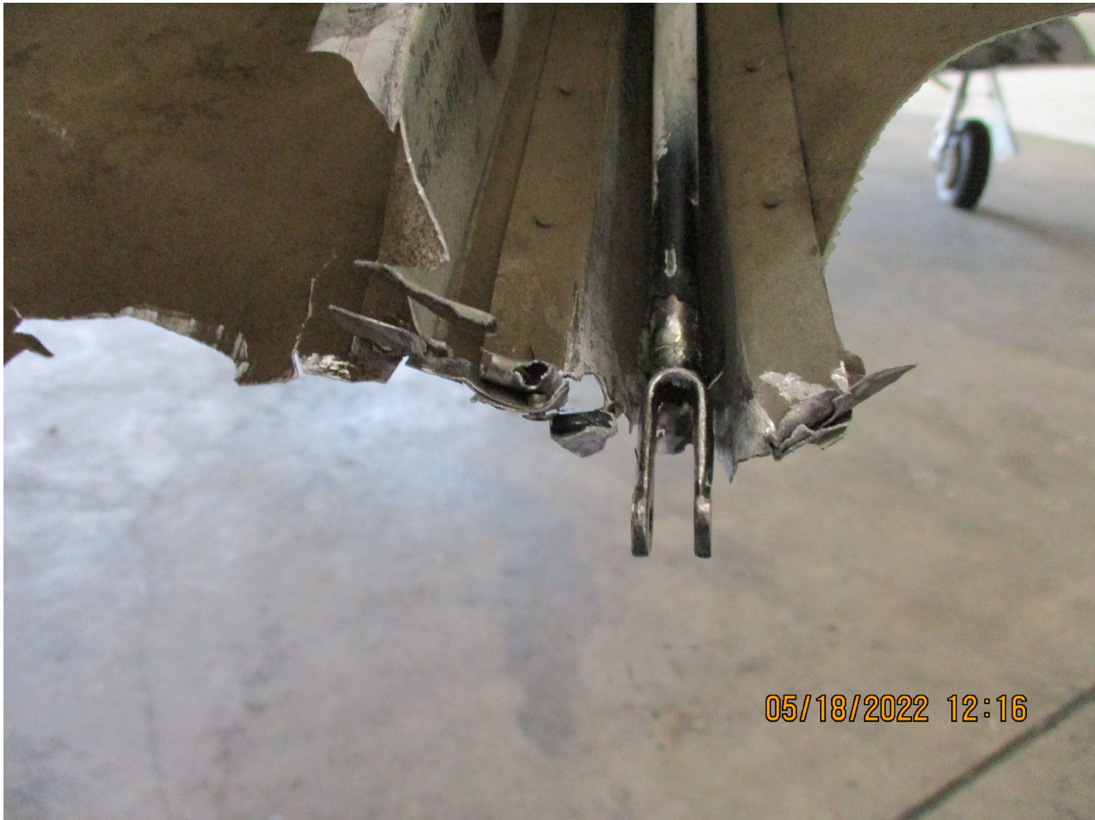
Photograph 4 - Elevator trim push-pull tube with hardware missing (Courtesy of FAA)
