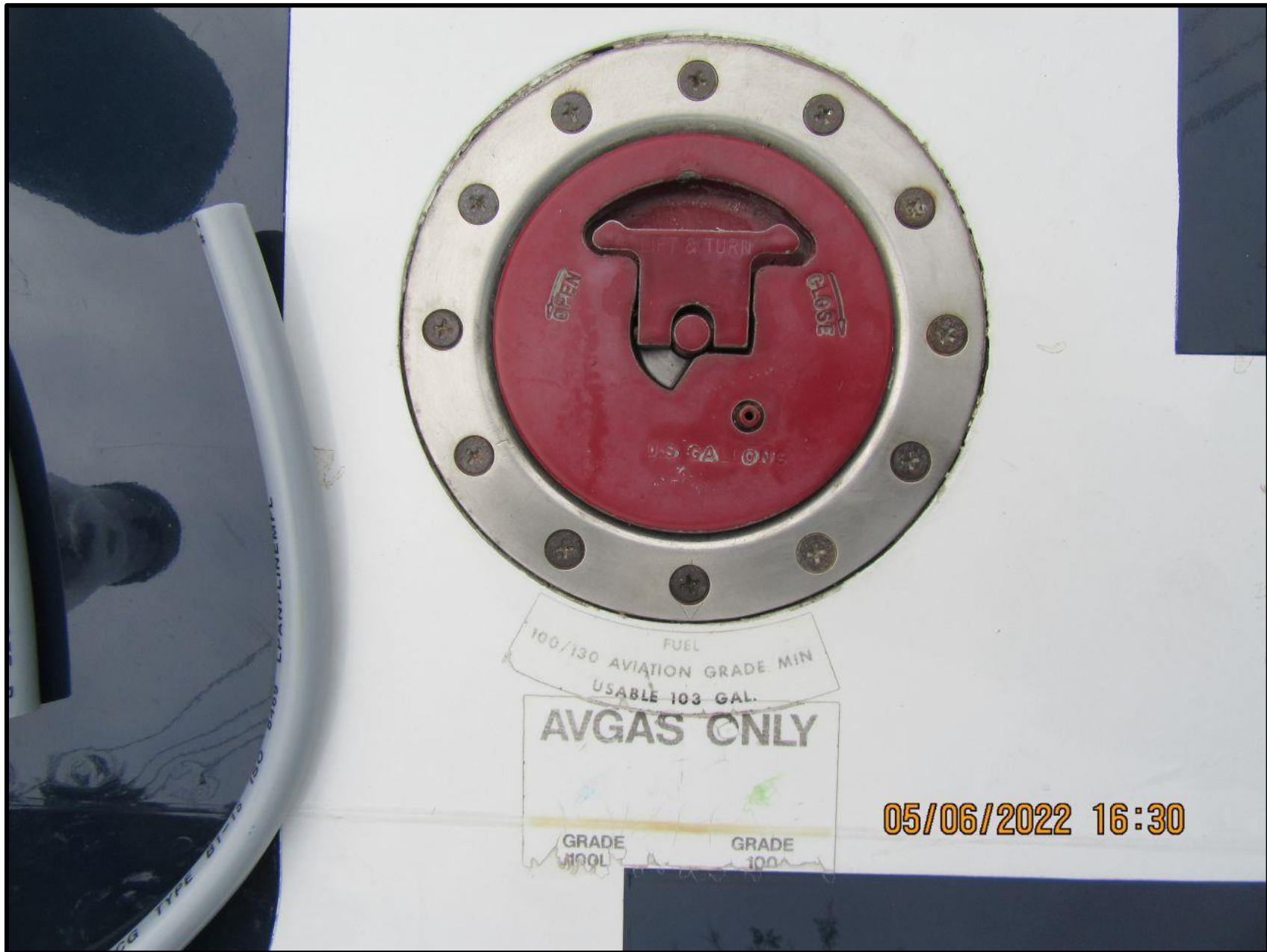
Photo 3 – Right Wing Fuel Filler Port (FAA Photo)
