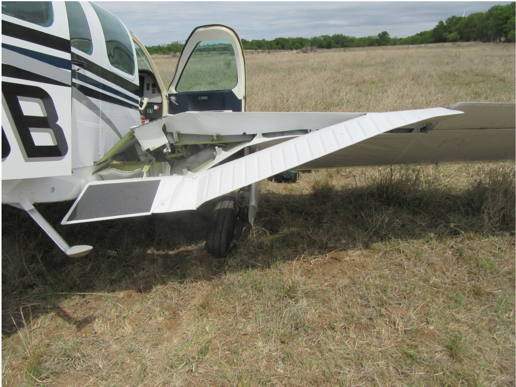
Photo 4 – View of the substantial damage sustained to the right wing at the accident site (courtesy of the Federal Aviation Administration).
