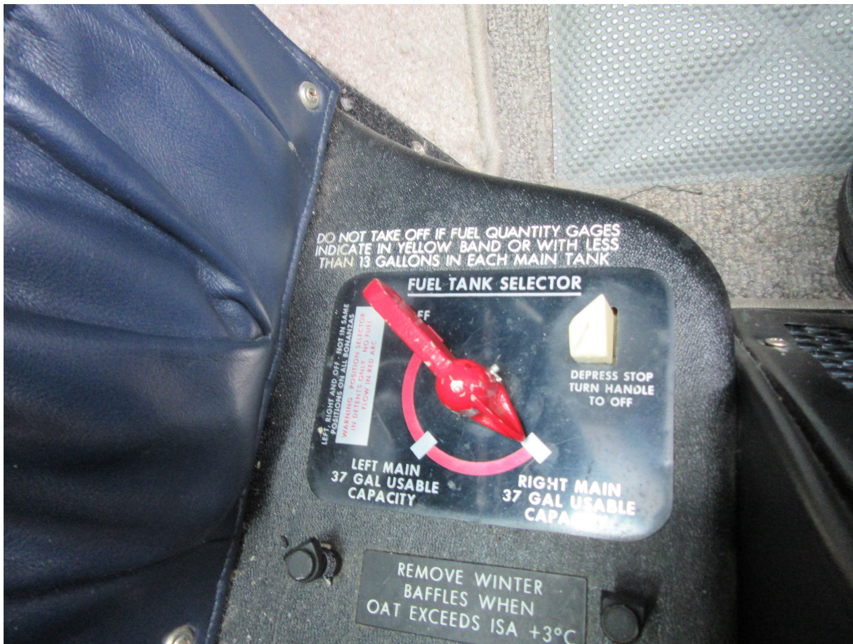
Photo 6 – View of the fuel tank selector at the accident site (courtesy of the Federal Aviation Administration).
