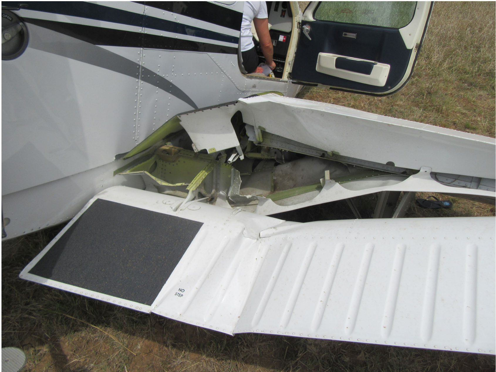
Photo 5 – Close up view of the substantial damage sustained to the right wing at the accident site (courtesy of the Federal Aviation Administration).
