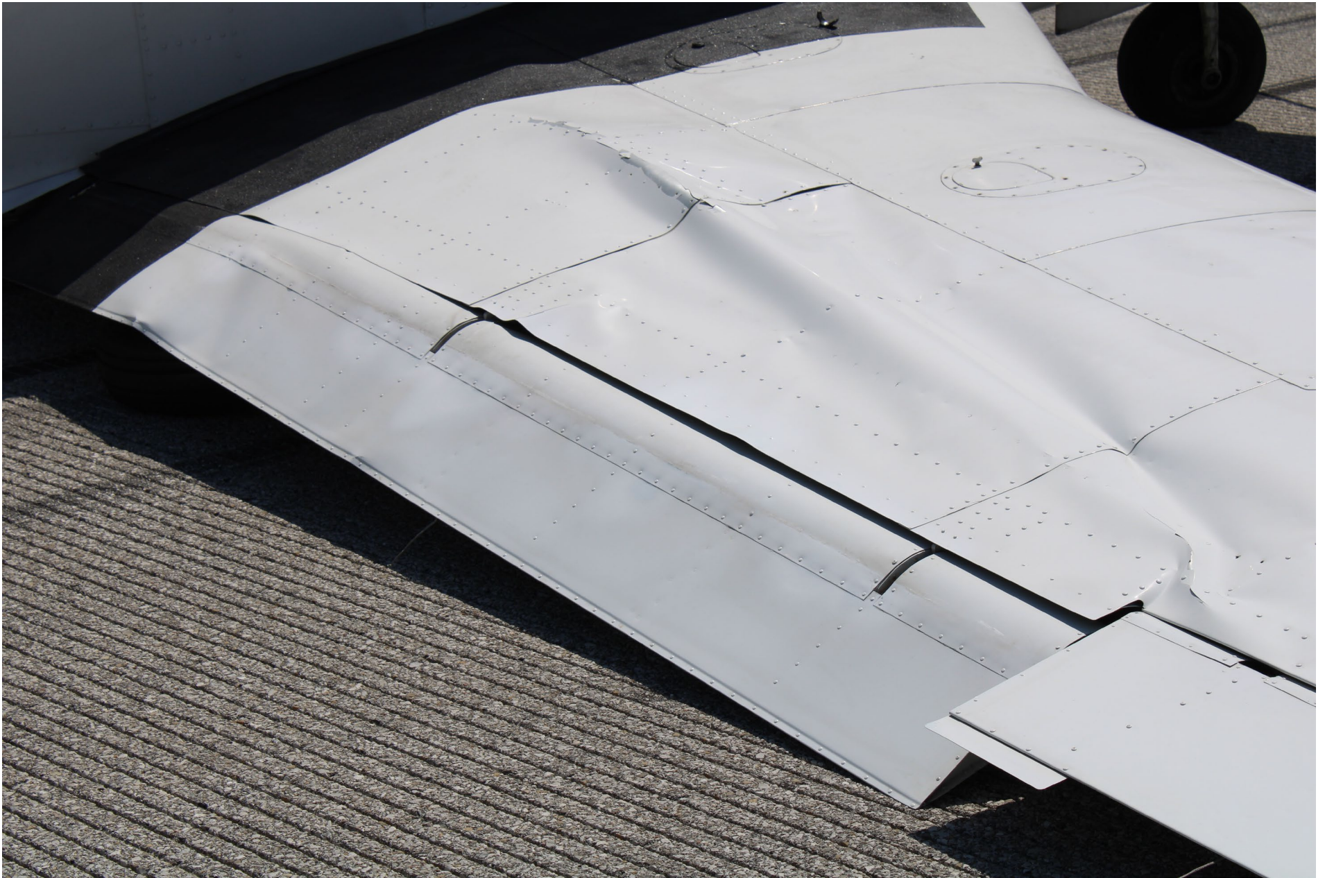
Photo 3 – Right wing damage
