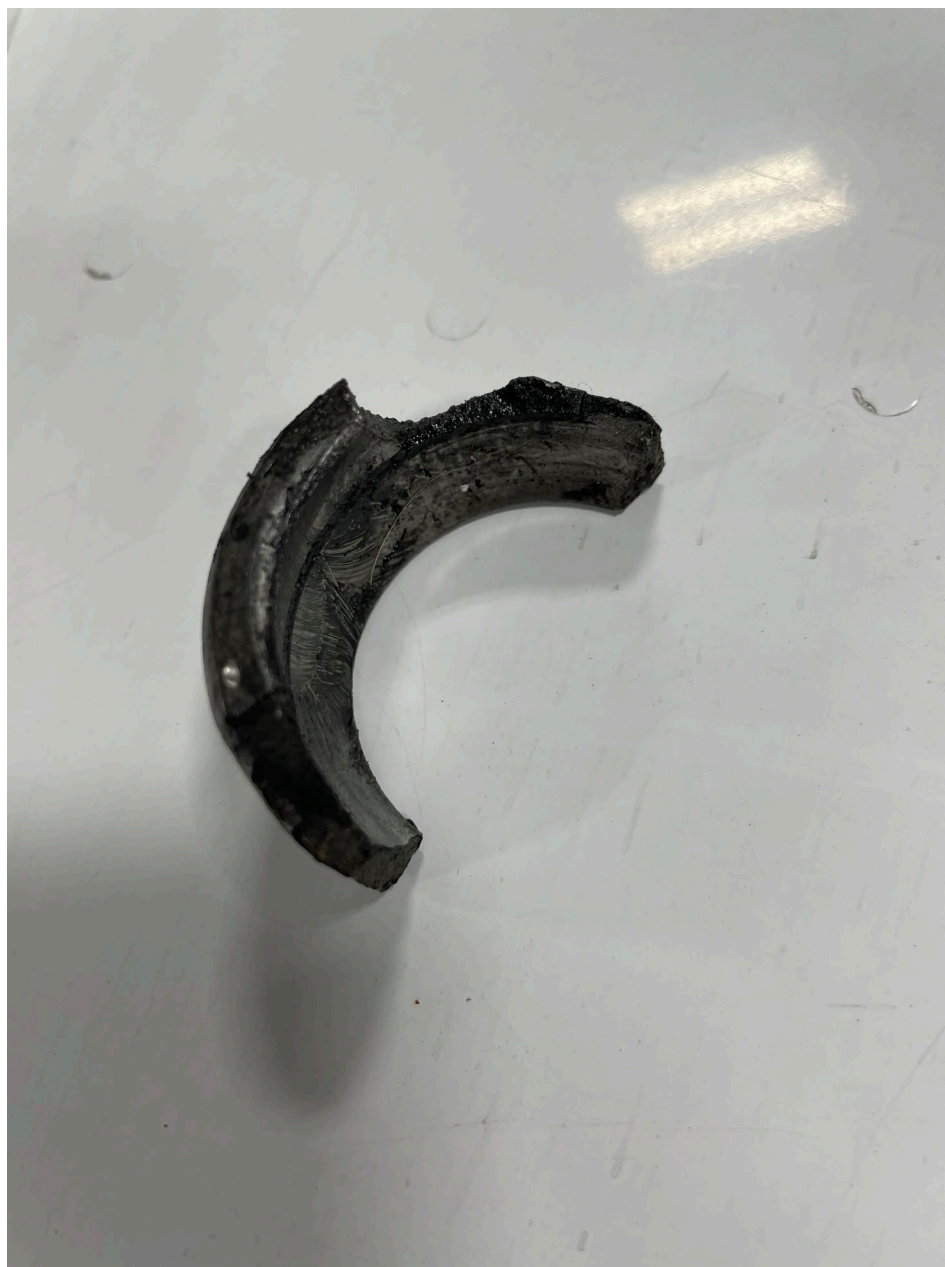
Photo 2 – Bearing found on runway – Courtesy of FAA
