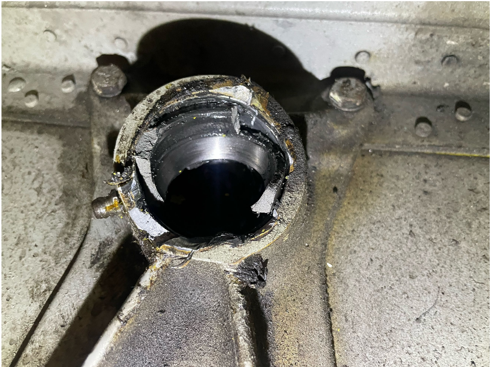
Photo 1 – Trunnion damage to right main landing gear - Photo courtesy of Federal Aviation Administration (FAA)
