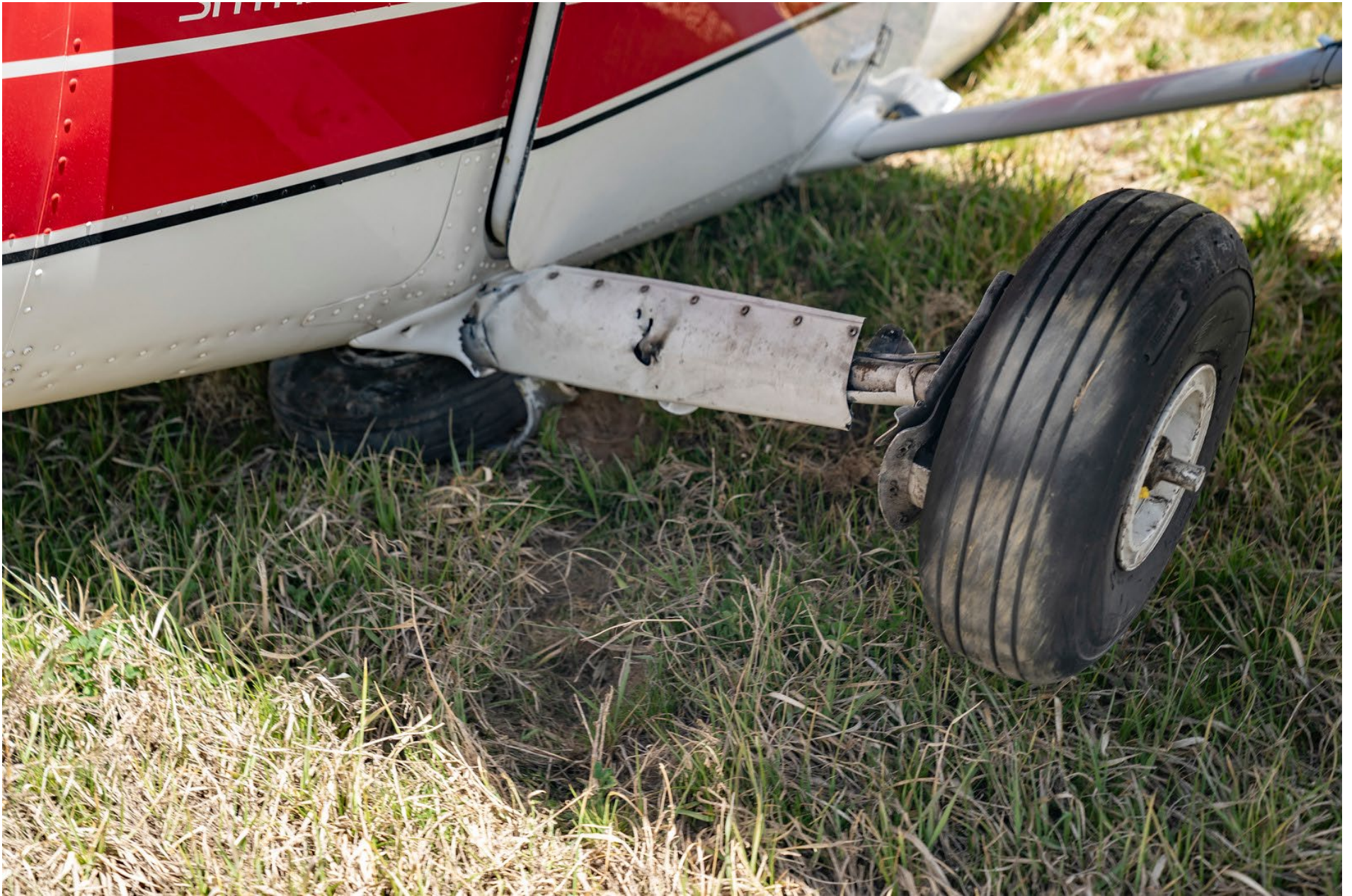
Photo 2 – Collapsed Landing Gear (Courtesy of South Metro Fire and Rescue)
