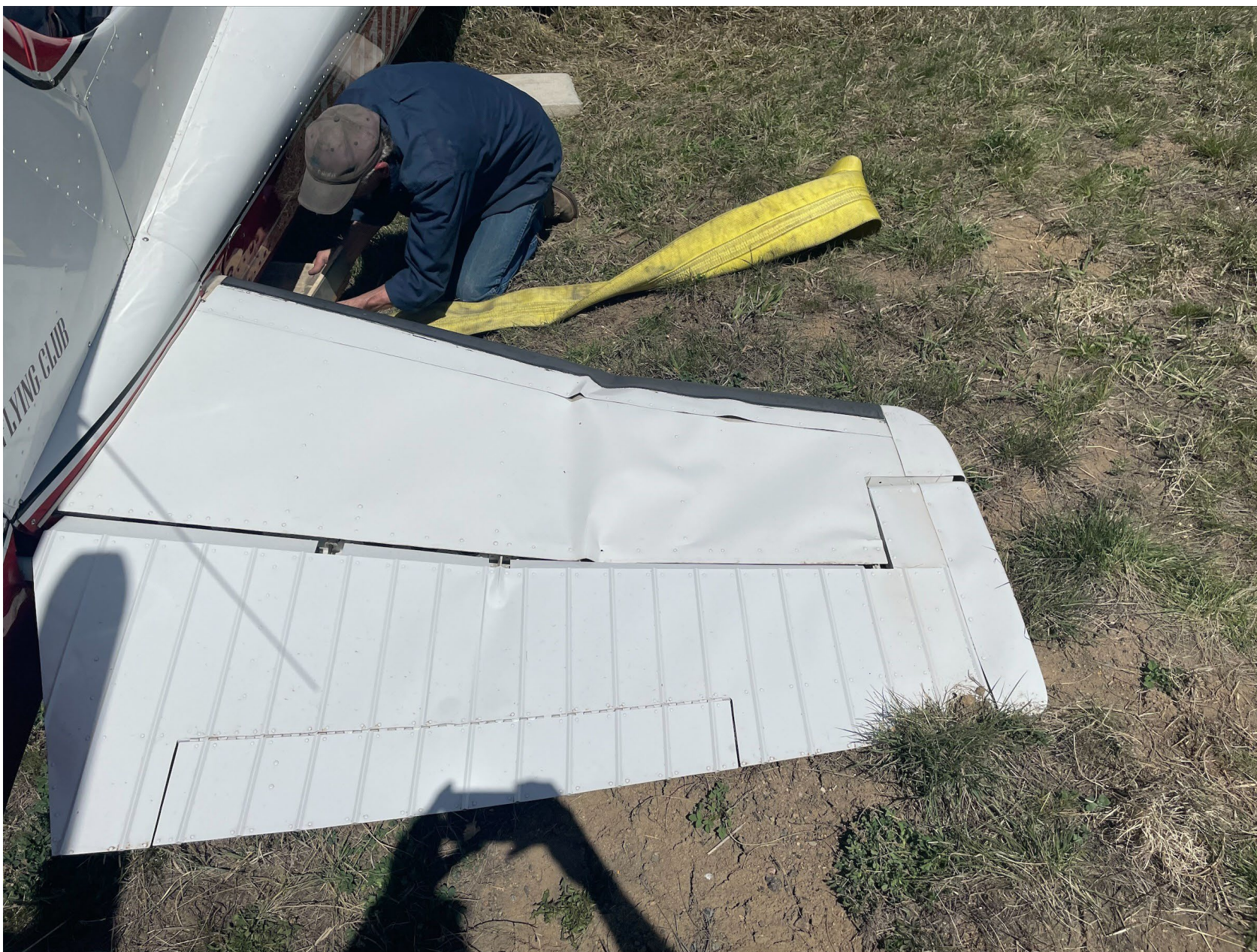
Photo 1 – Horizontal Stabilizer Damage (Courtesy of South Metro Fire and Rescue)
