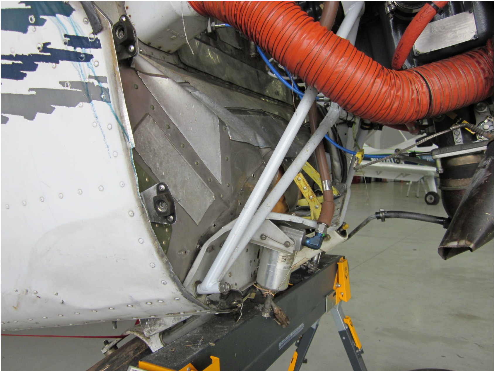
Photo 1 – Damage to Firewall and Fuselage (FAA Photo)
