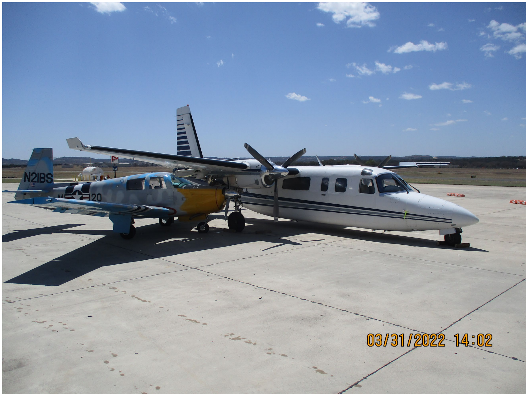
Photo 2 - N21BS Underneath the Right Wing of N25CE Side View (Source: FAA)
