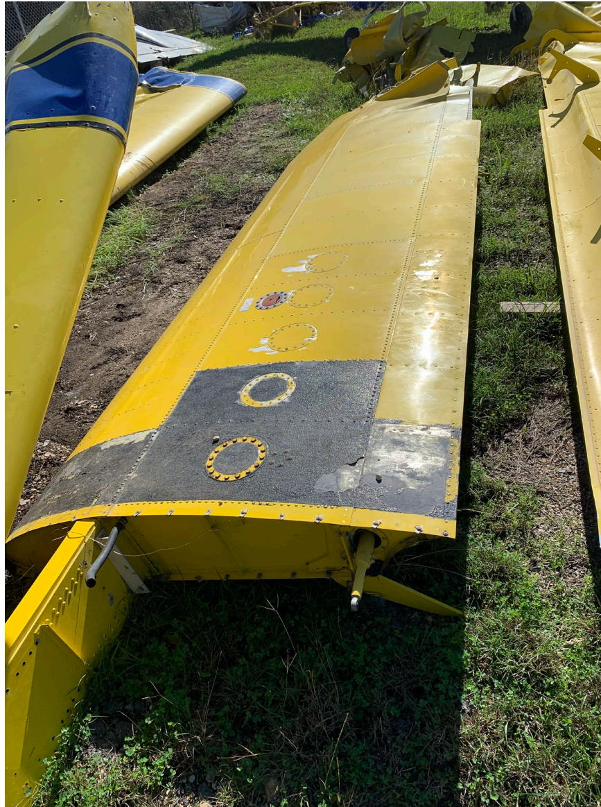
Photograph 3 - Right wing during postaccident examination (NTSB Photo)
