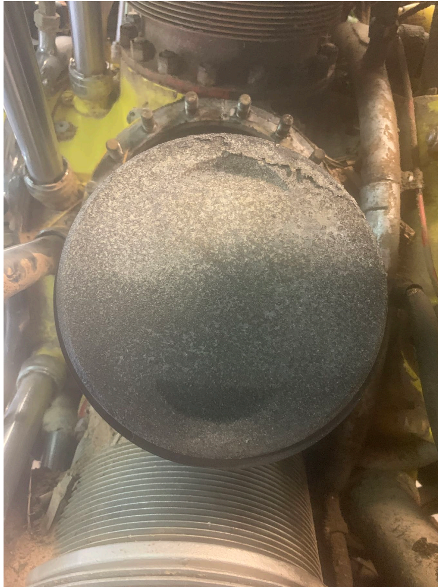
Photograph 6 - No. 8 piston during postaccident examination (NTSB Photo)
