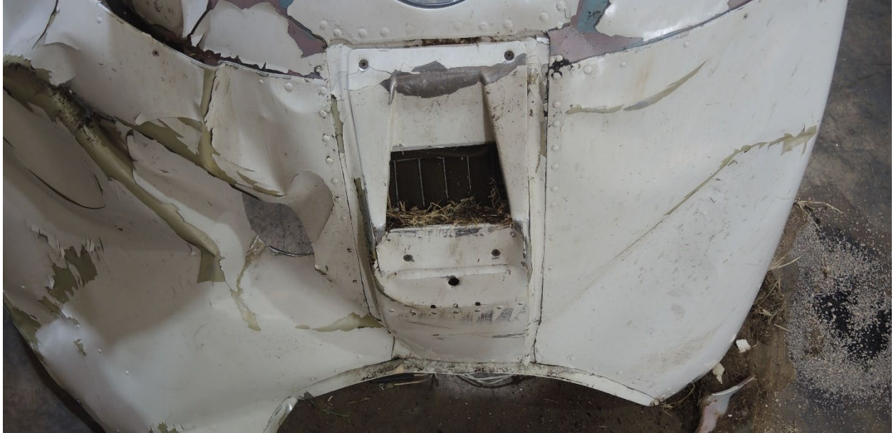
The lower cowl induction air filter was in place and undamaged with dirt and organic debris at the bottom of the filter element.
