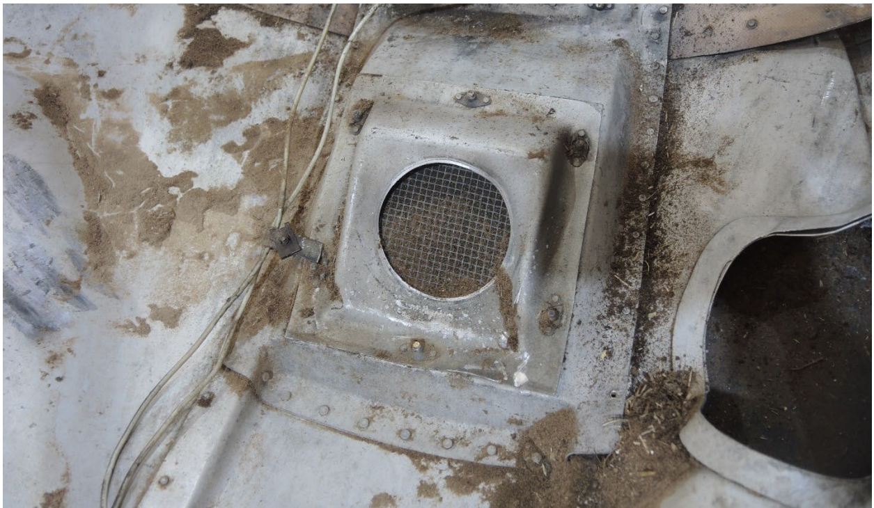
The induction air filter screen was in place and undamaged with dirt and organic debris in the filter and screen. The hose from the filter to the carburetor inlet was clear and only contained a small amount of dirt.
