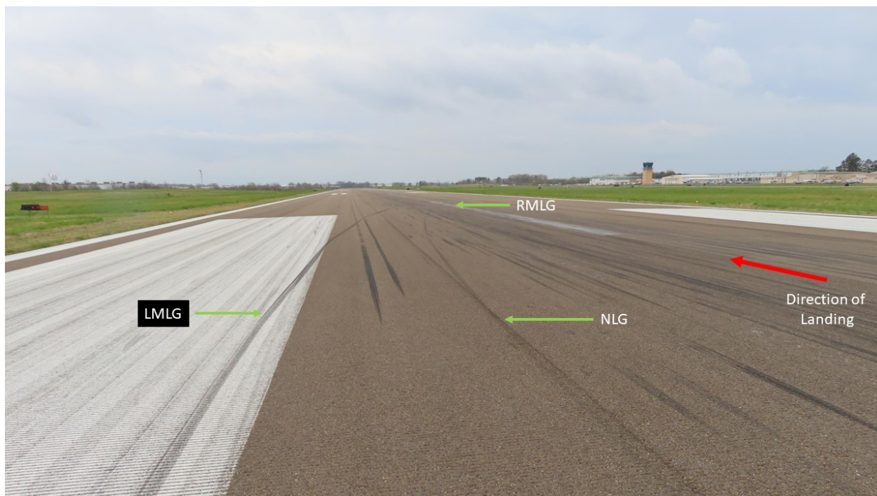
Figure 4. Runway markings (Source: Piper Aircraft, annotated by NTSB).
