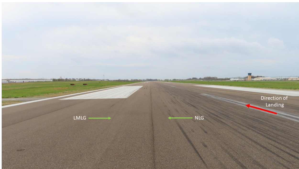
Figure 3. Initial touchdown runway markings (Source: Piper Aircraft, annotated by NTSB).
