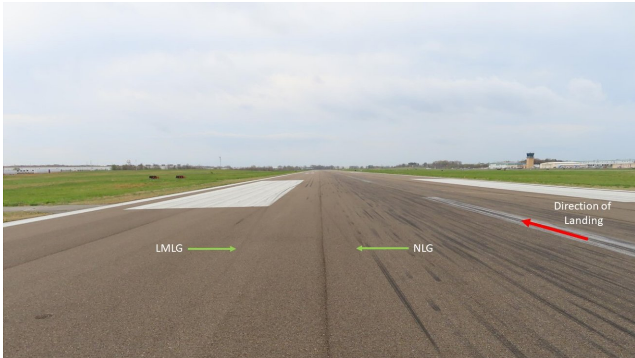
Figure 3. Initial touchdown runway markings (Source: Piper Aircraft, Inc., annotated by NTSB)
