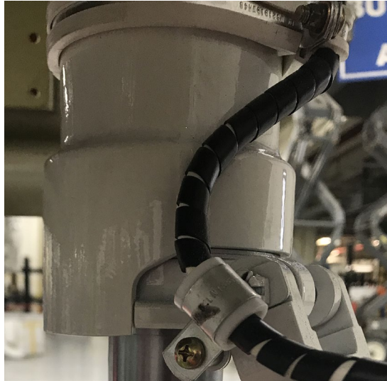
Figure 7. M600 right turn mechanical stop between trunnion and strut just prior to engagement
