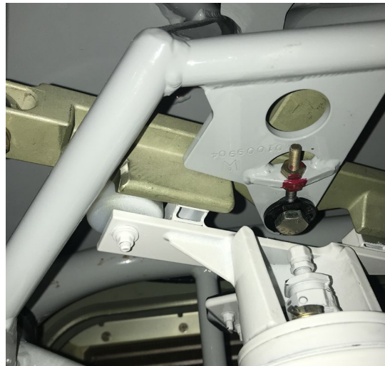
Figure 8. M600 left turn mechanical stop between engine mount and steering arm just prior to engagement
