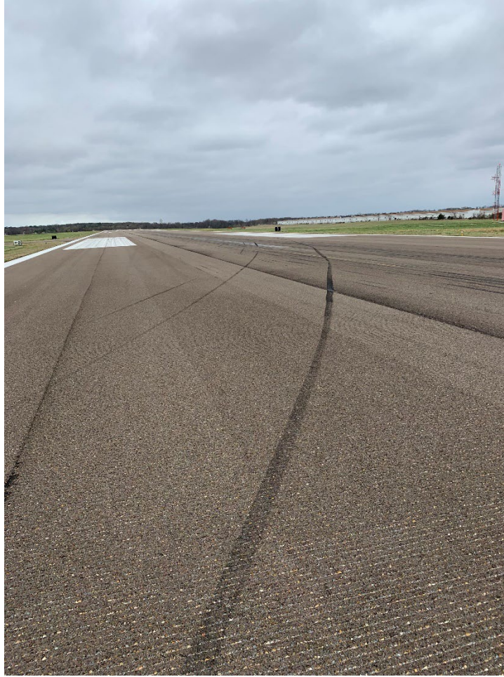
Figure 5: Tire Marks on the Runway Surface (looking toward the approach end of the runway)
