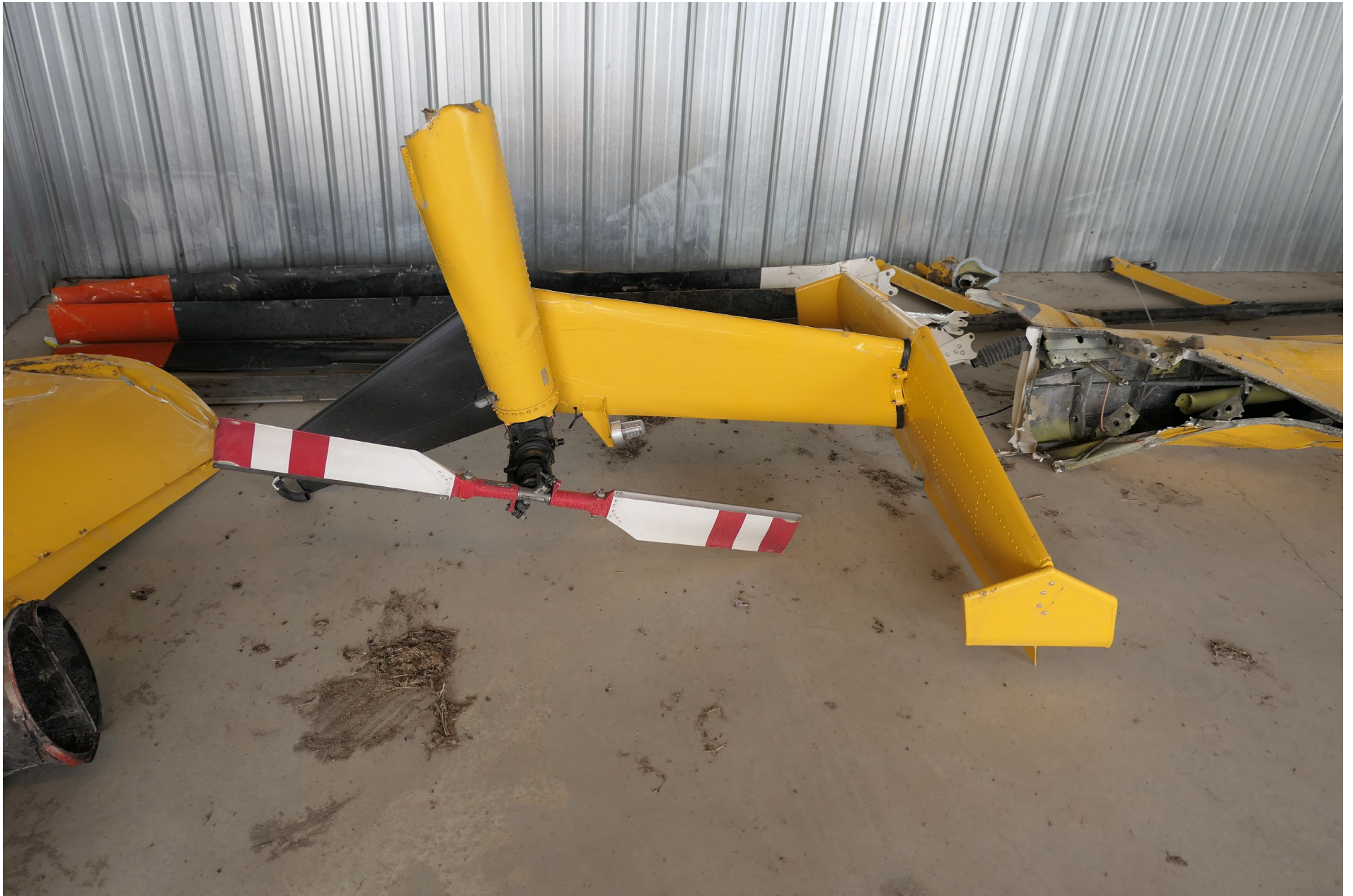
Photo 8 – View of the tail rotor system after it was recovered from the accident site (courtesy of MD Helicopters).
