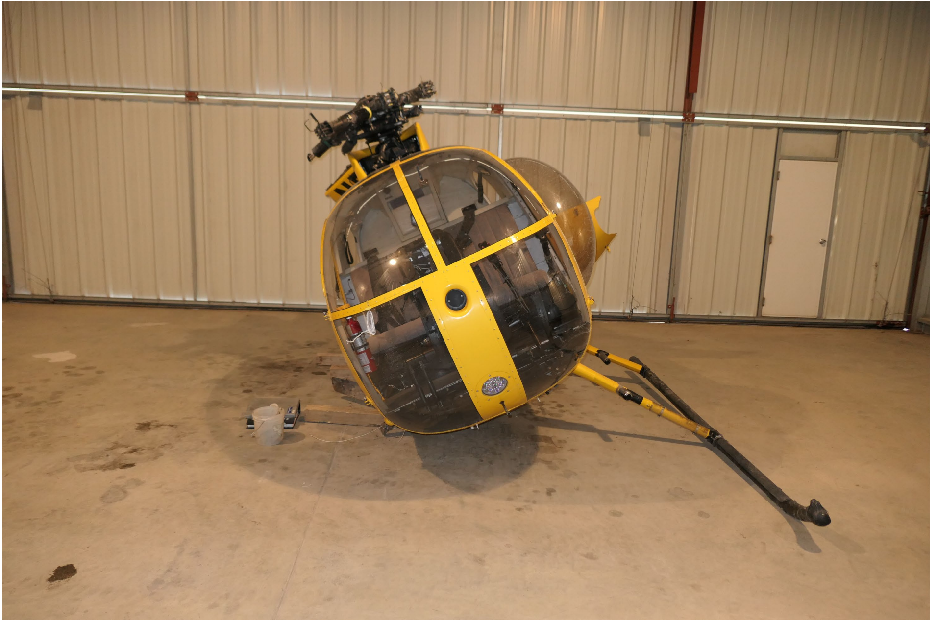
Photo 3 – View of the front of the fuselage after it was recovered from the accident site (courtesy of MD Helicopters).
