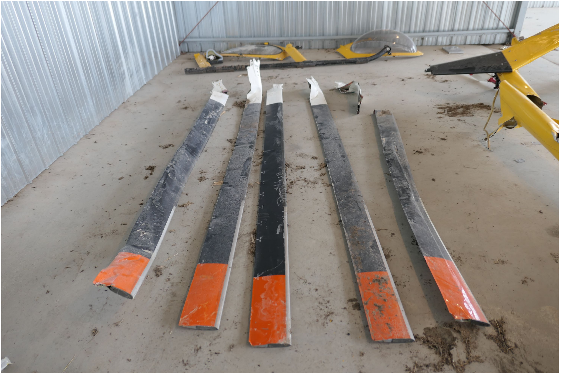
Photo 6 – View of the main rotor blades after they were recovered from the accident site (courtesy of MD Helicopters).
