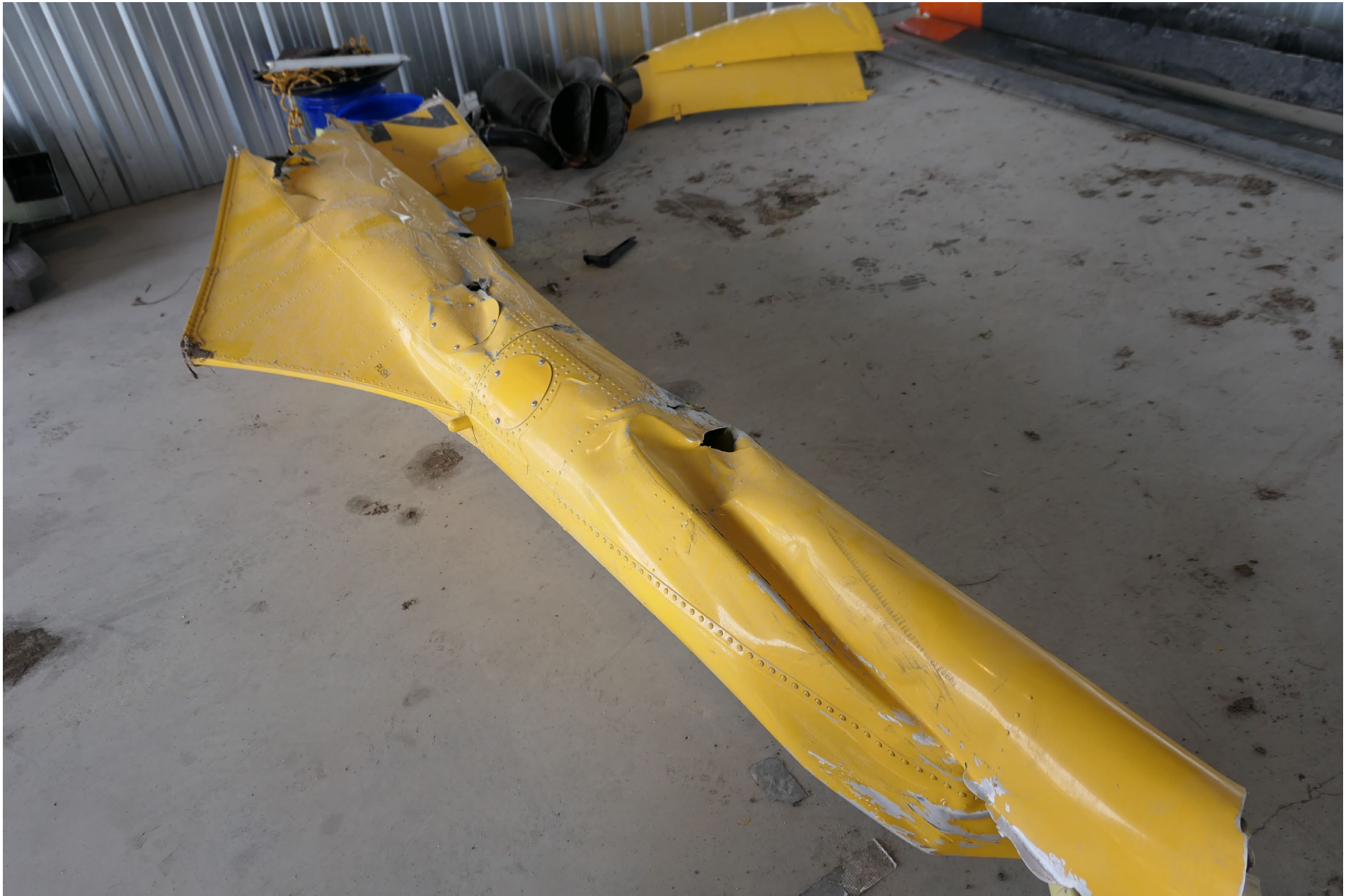
Photo 7 – View of the tail boom after it was recovered from the accident site (courtesy of MD Helicopters).
