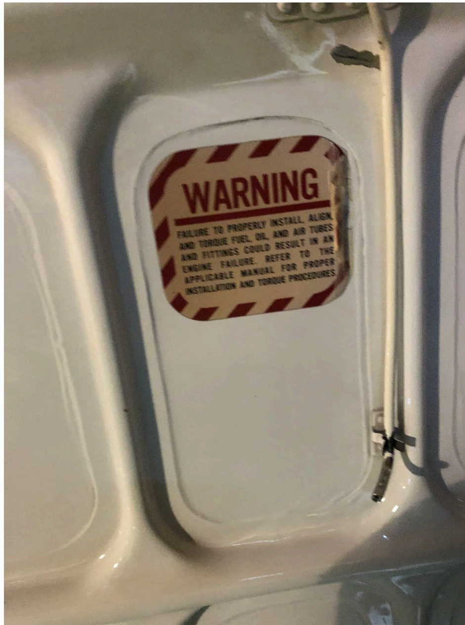
Photo 10 – View of the required placard in the engine compartment of the accident helicopter (courtesy of Winco Powerline Services).
