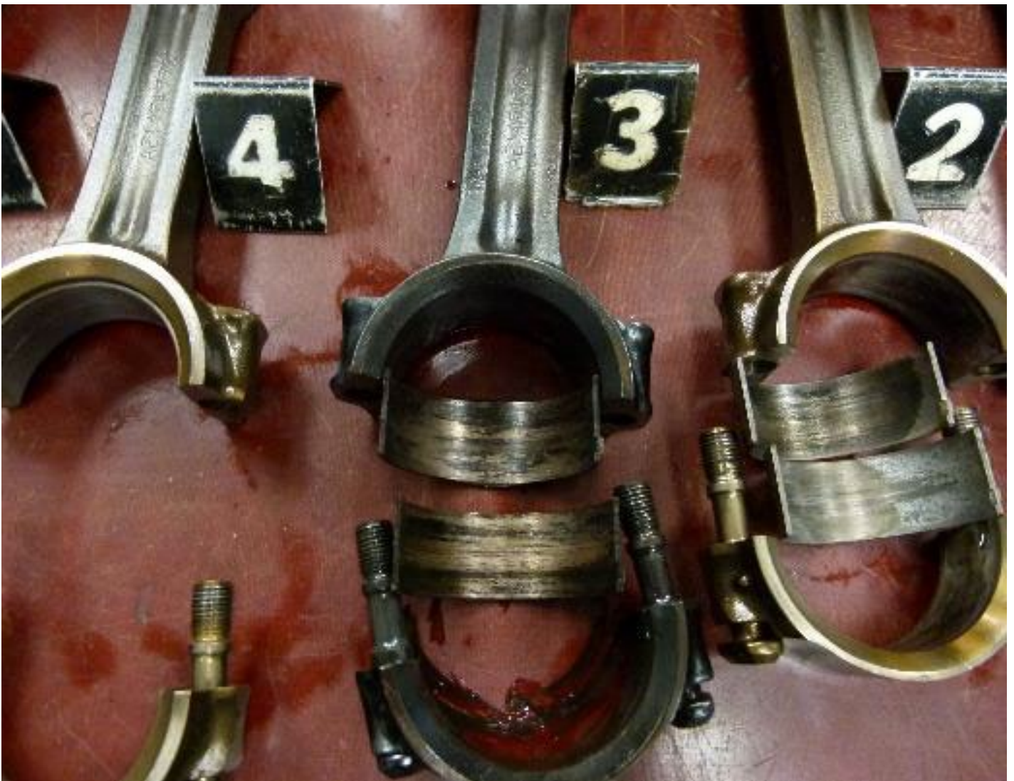
Photo 3 Closeup View of #3 Connecting Rod & Bearing Showing Thermal Distress
