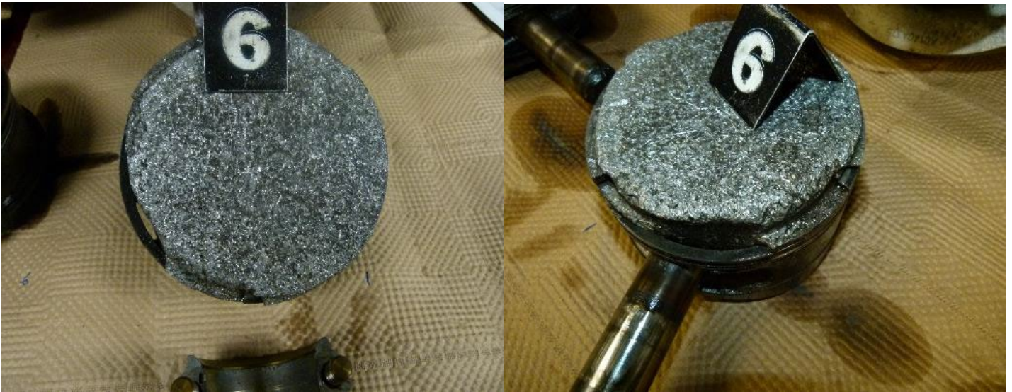
Photo 2 Closeup Views of #6 Piston Damage
