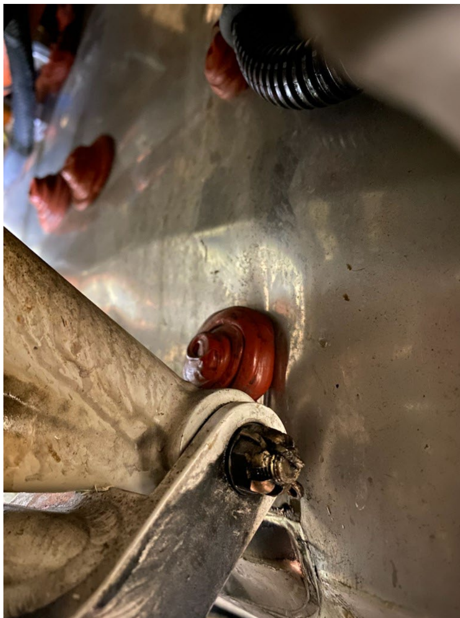
Photo 2 – Substantial Damage to Firewall (Source: FAA)
