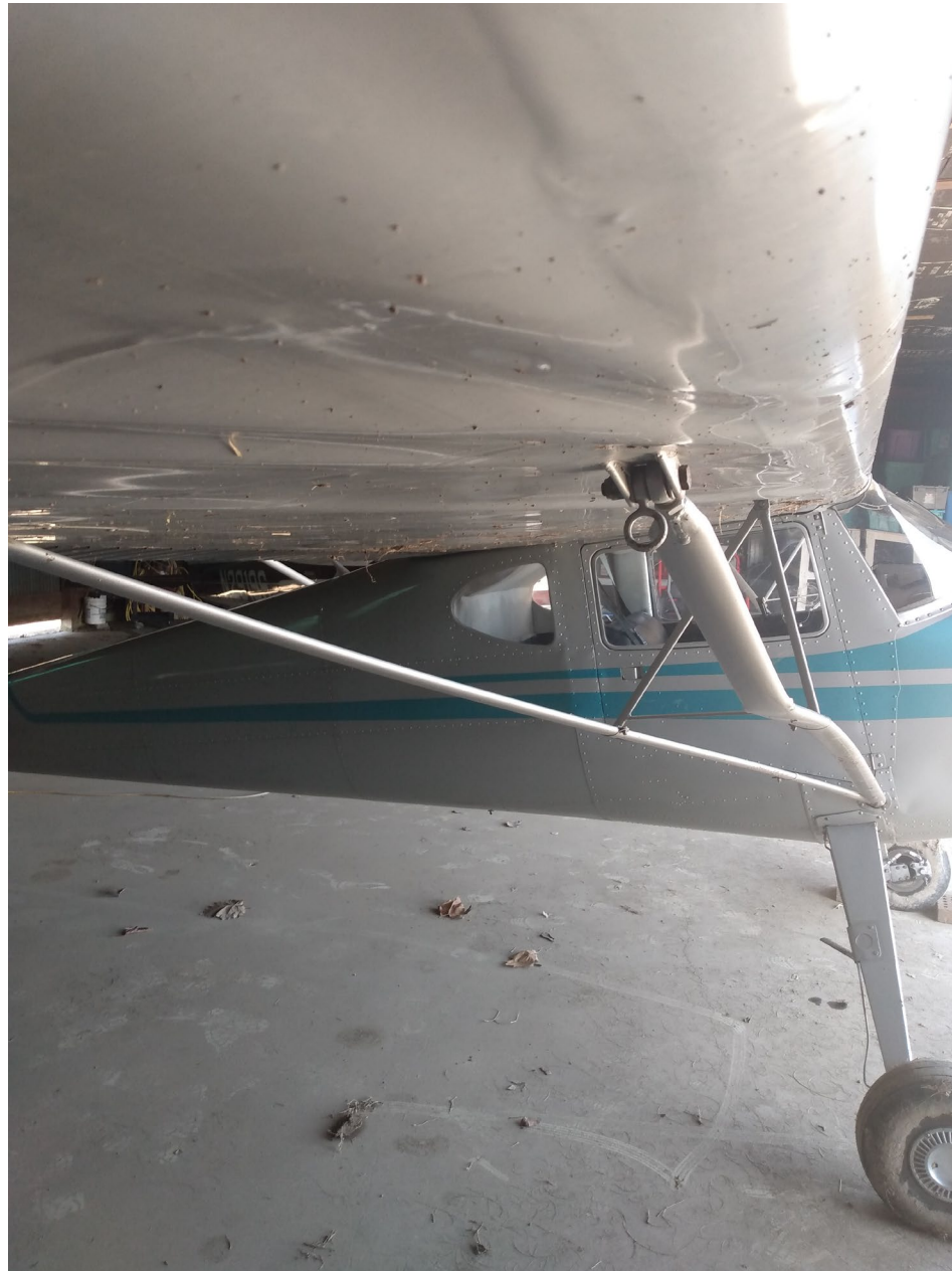
Photo 1 – View of bent wing and wing strut (Photo provided by FAA)
