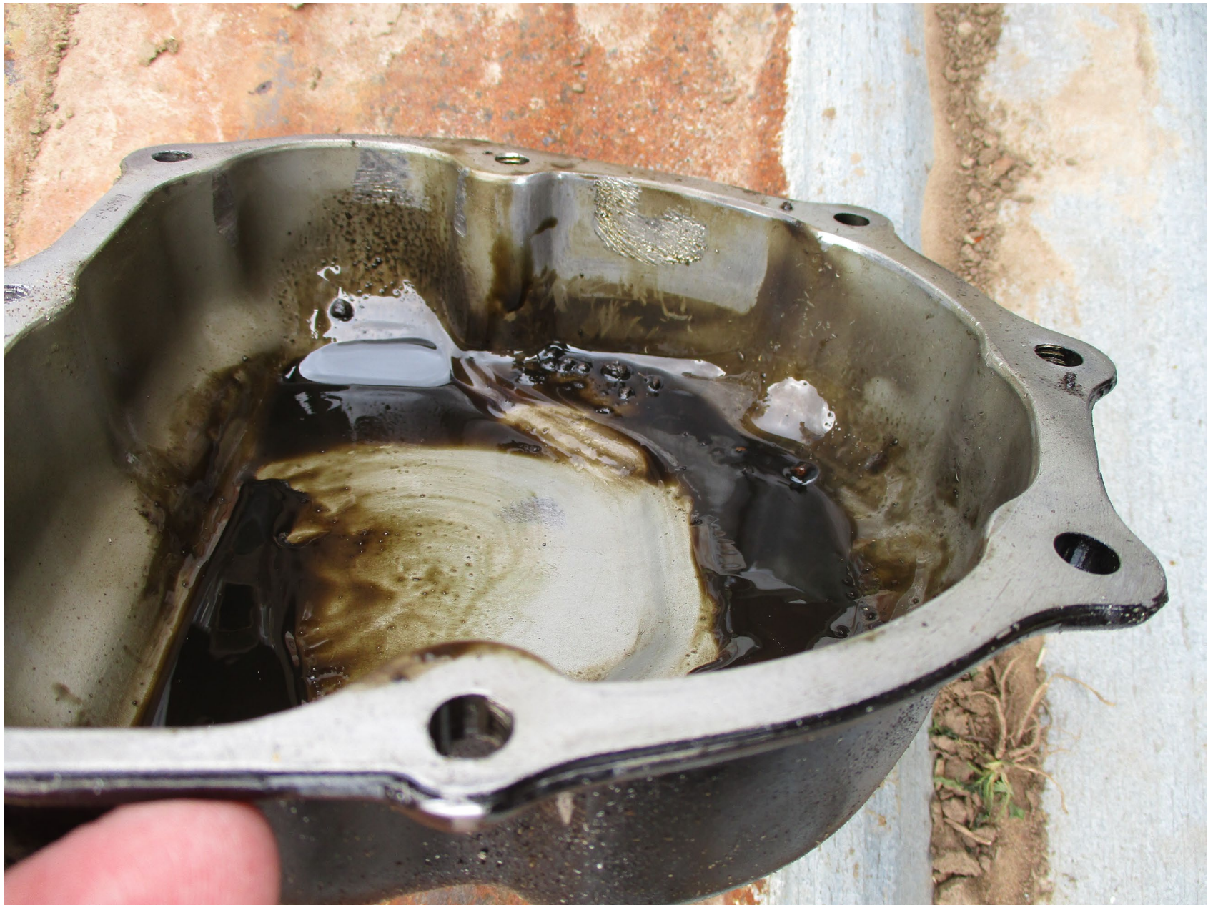
Photo 7 – Contaminated oil in rocker cover (FAA Photo)
