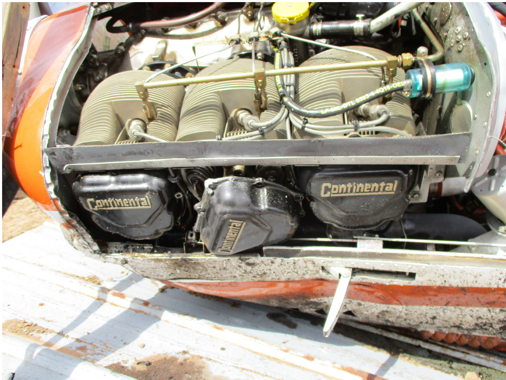
Photo 4 – View of engine left side showing loose No. 4 rocker cover (FAA Photo)
