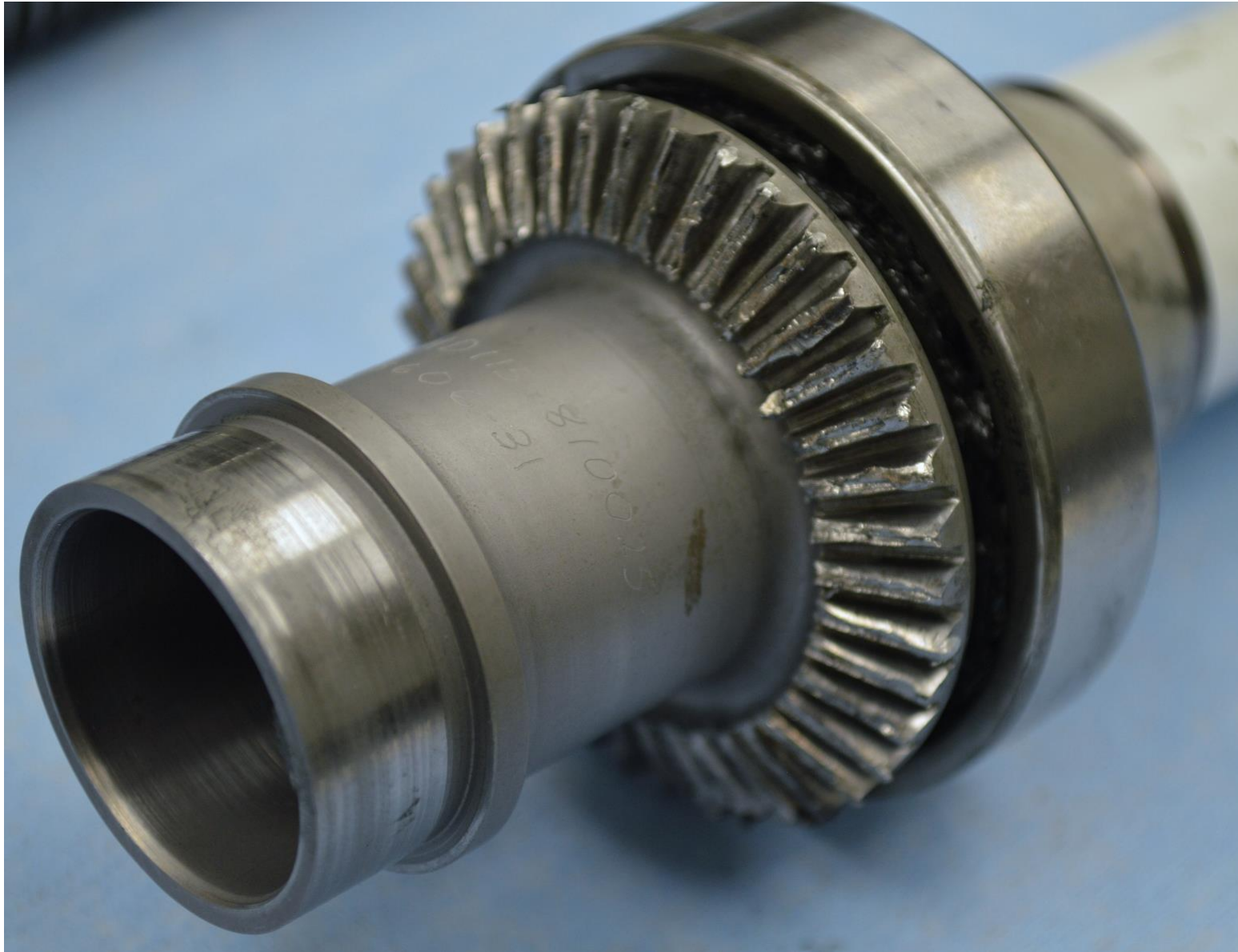
Figure 20: 115-810025-1 Driven Gear with damaged Gear Teeth. (Mag x2)
