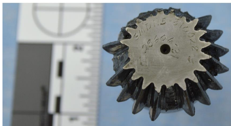
Figure 12: 115-810028-3 Drive Gear and Broken Gear Teeth
