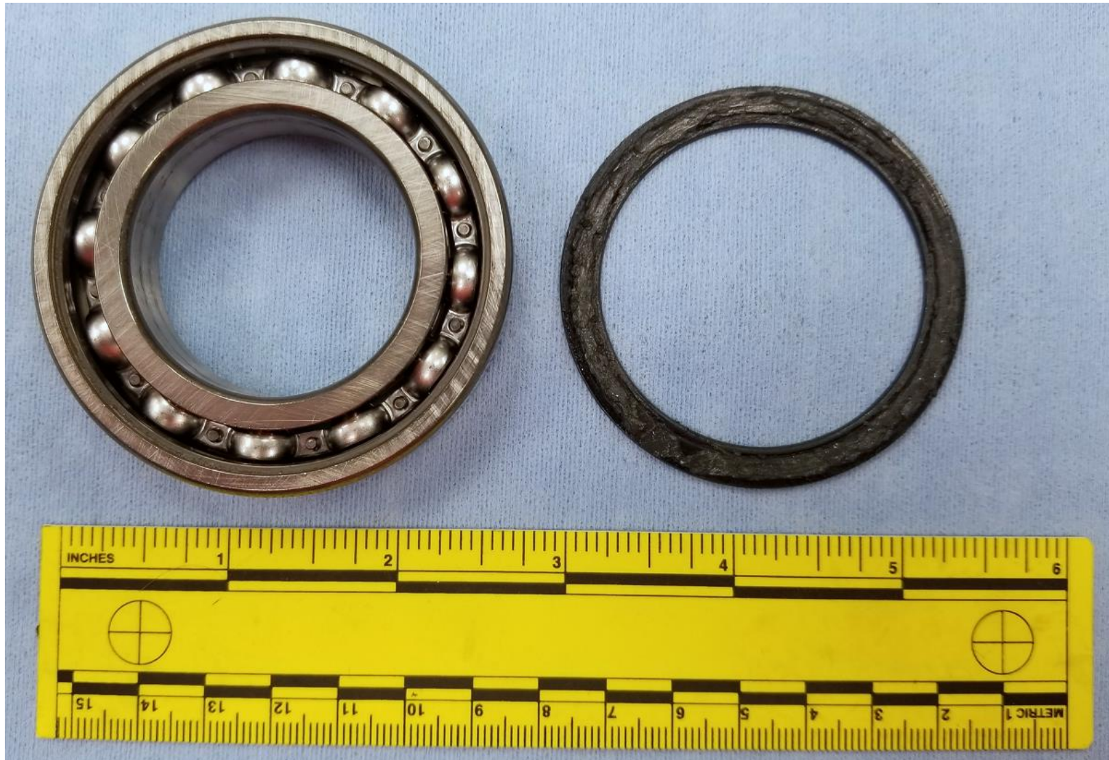
Figure 26: Upper Bearing removed from housing. (Mag x0.6)
