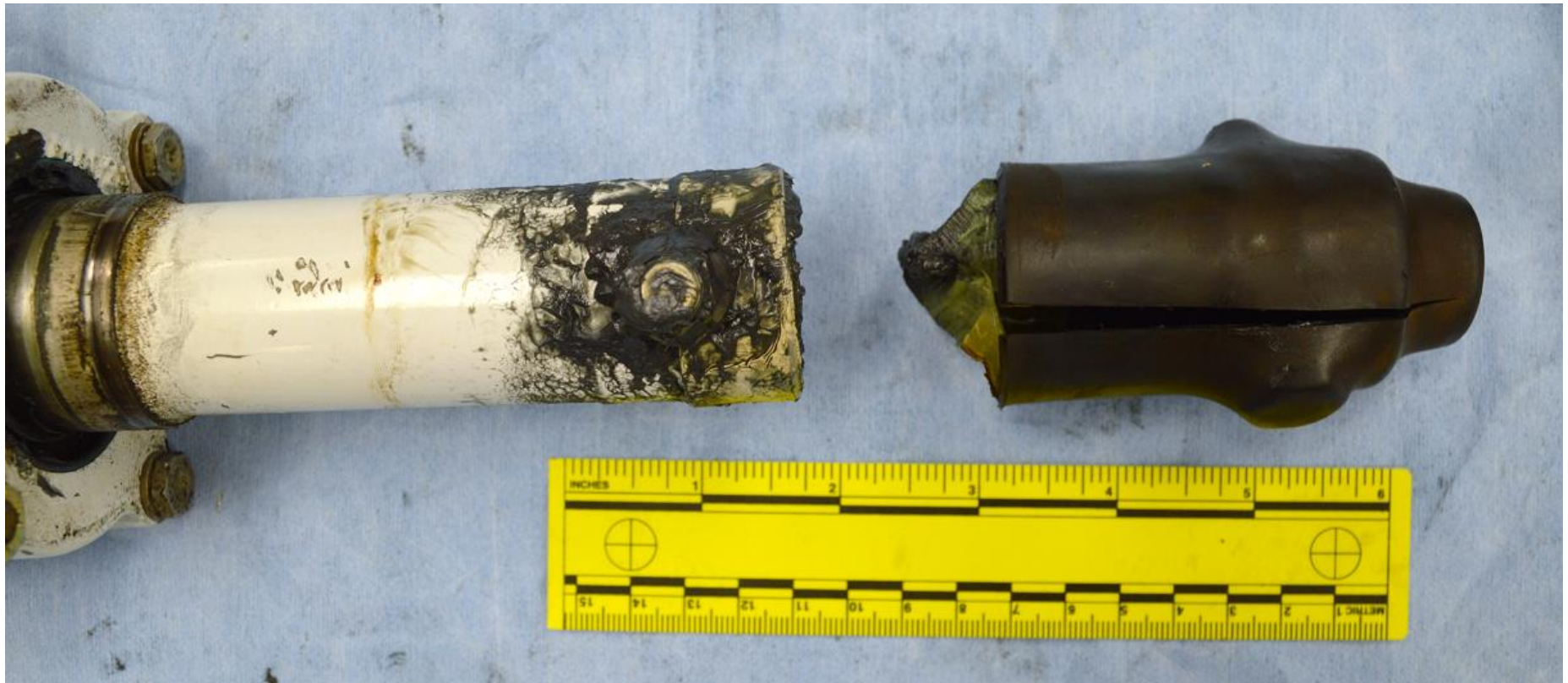
Figure 7: Boot Removal (Mag x0.75)
