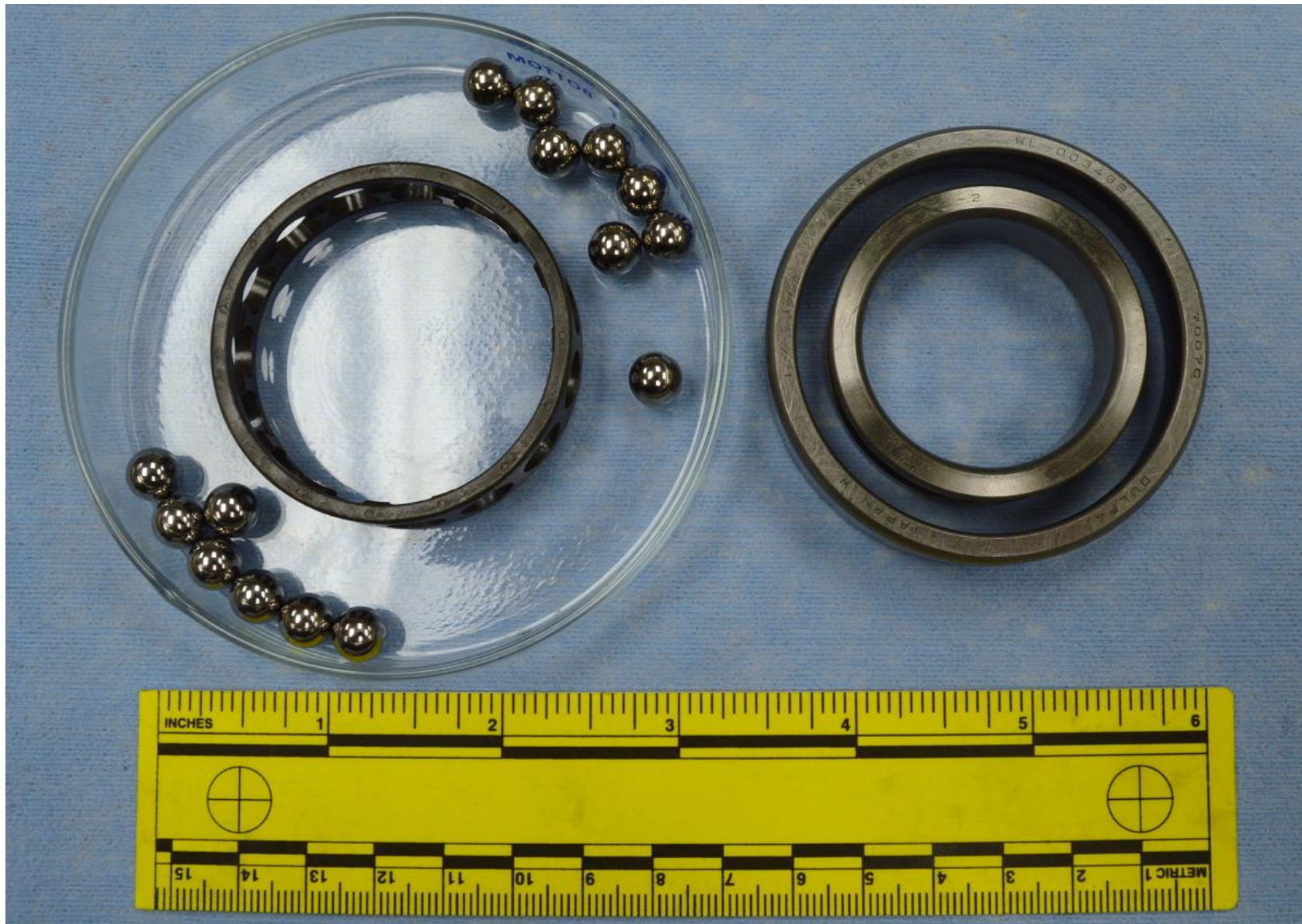
Figure 25: Lower Bearing removed from housing. (Mag x0.6)
