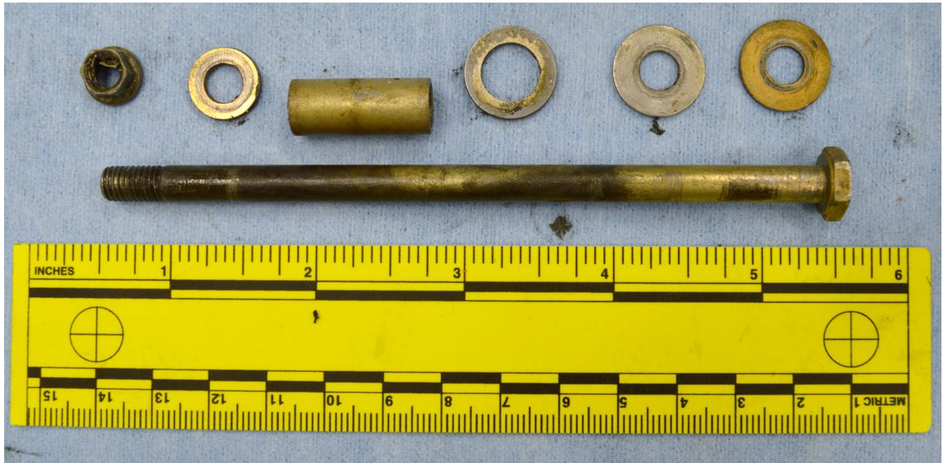
Figure 6: Pivot Bolt for Brake Assembly (Mag x1.5)
