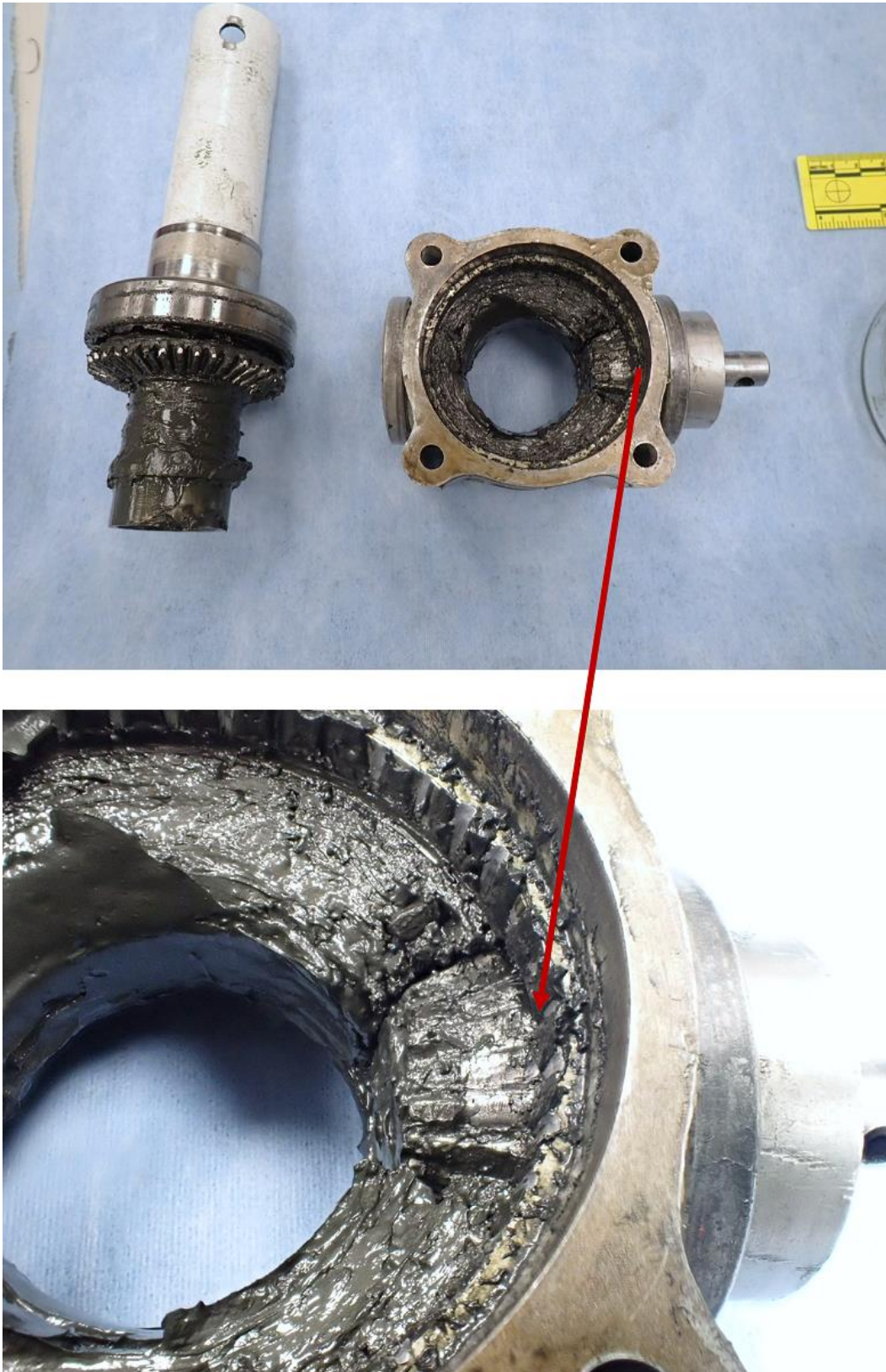
Figure 10: Housing with grease after removal of screw housing and upper bearing
