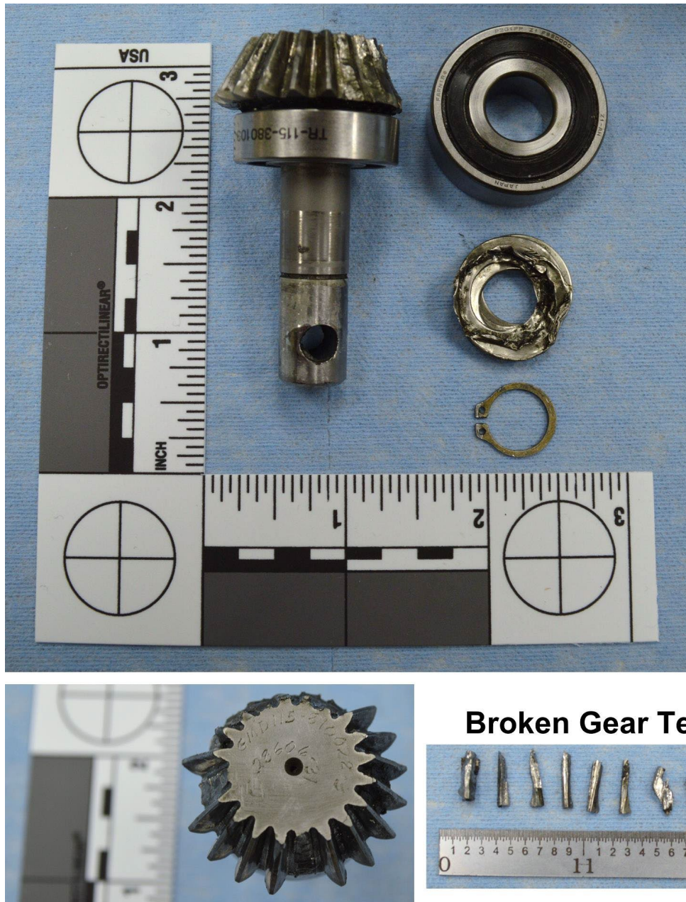
Figure 4. 115-810028-3 Pinion/Drive Gear and Broken Gear Teeth.
