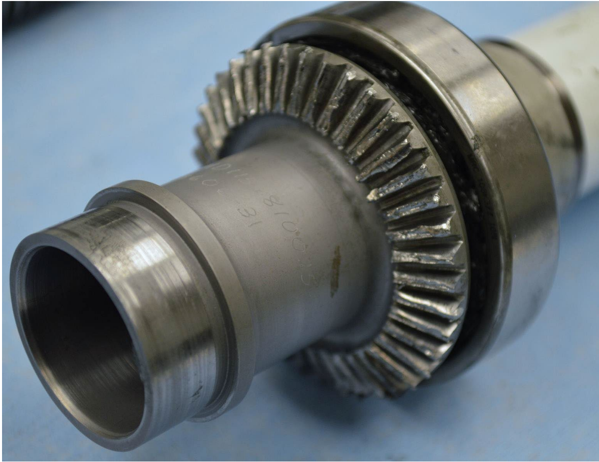
Figure 7. 115-810025-1 Driven Gear with damaged Gear Teeth.
