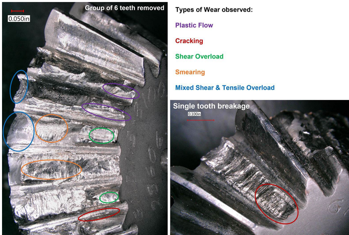
Figure 6. Different Types of Wear Visible on Pinion/Drive Gear Where Teeth are Missing.
