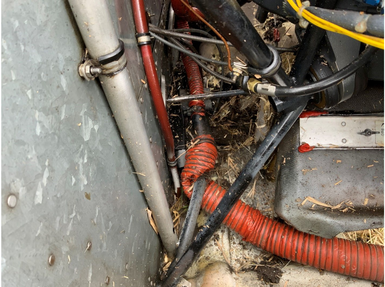
Photo 2: Bent Engine Mount and Ducting (Source: Federal Aviation Administration)
