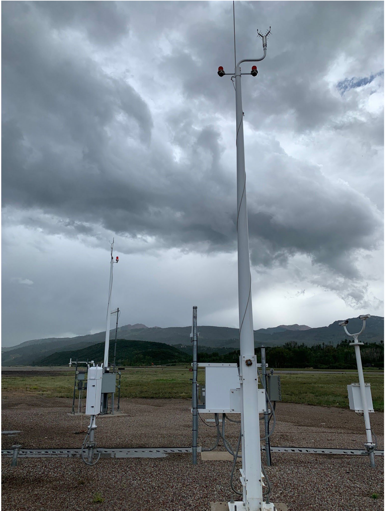
Figure 6. Wind sensors for both ASOS (foreground) and SAWS.
