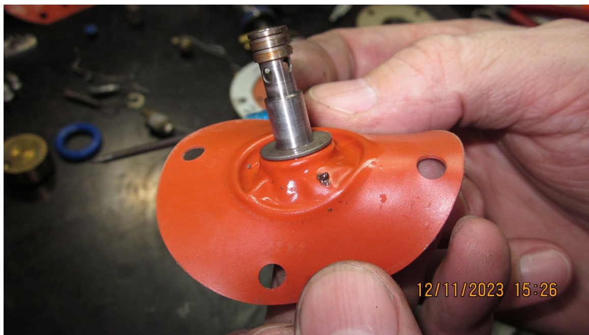
Photograph 3 - Fuel Divider Contaminant (Courtesy of FAA)
