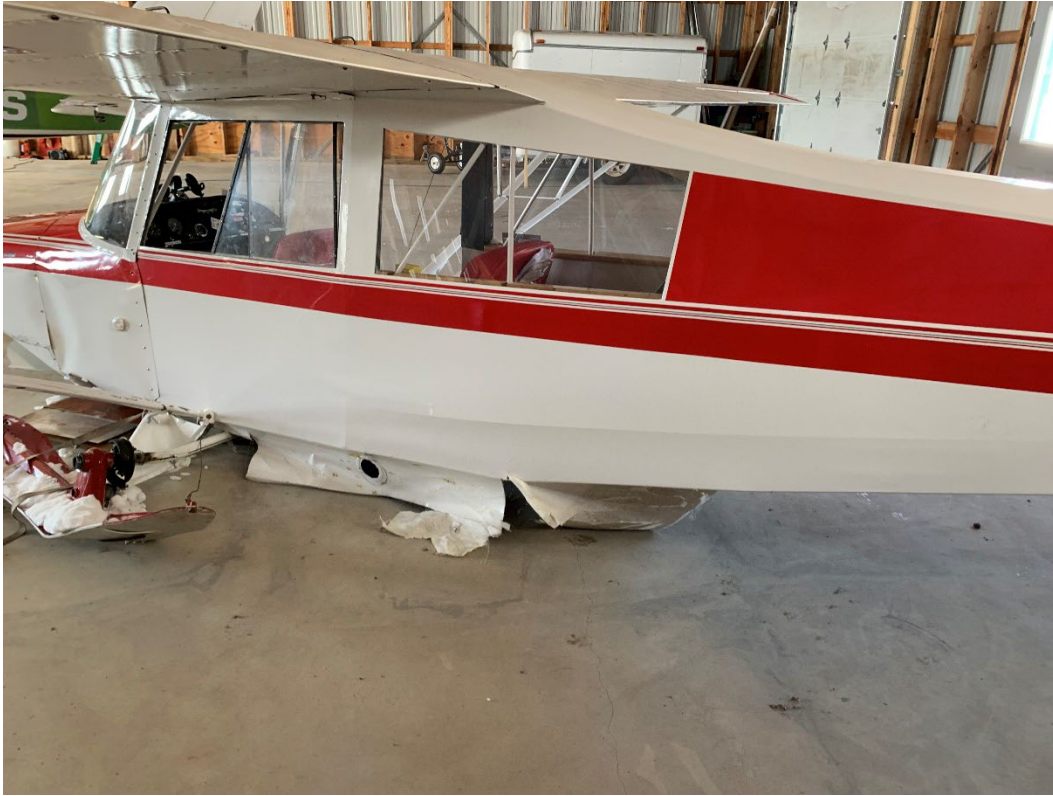
Figure 3: Lower Fuselage Damage
