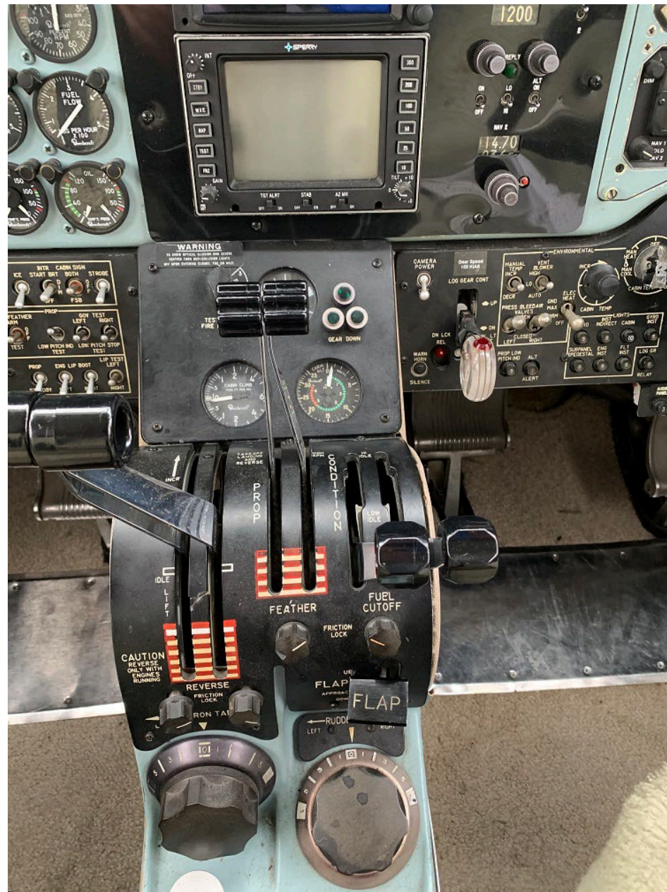
Photo 4 – Cockpit Control Pedestal (Source: FAA)
