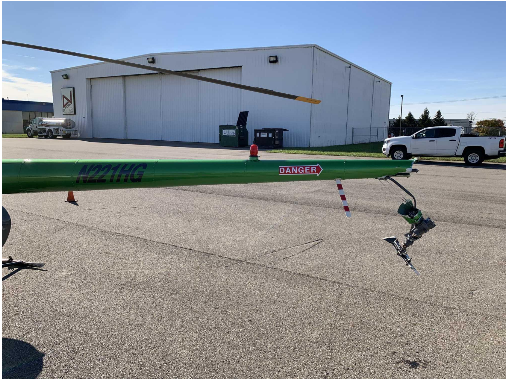
Photo 2 – Aft Tail Boom and Tail Rotor Gear Box (FAA Photo)
