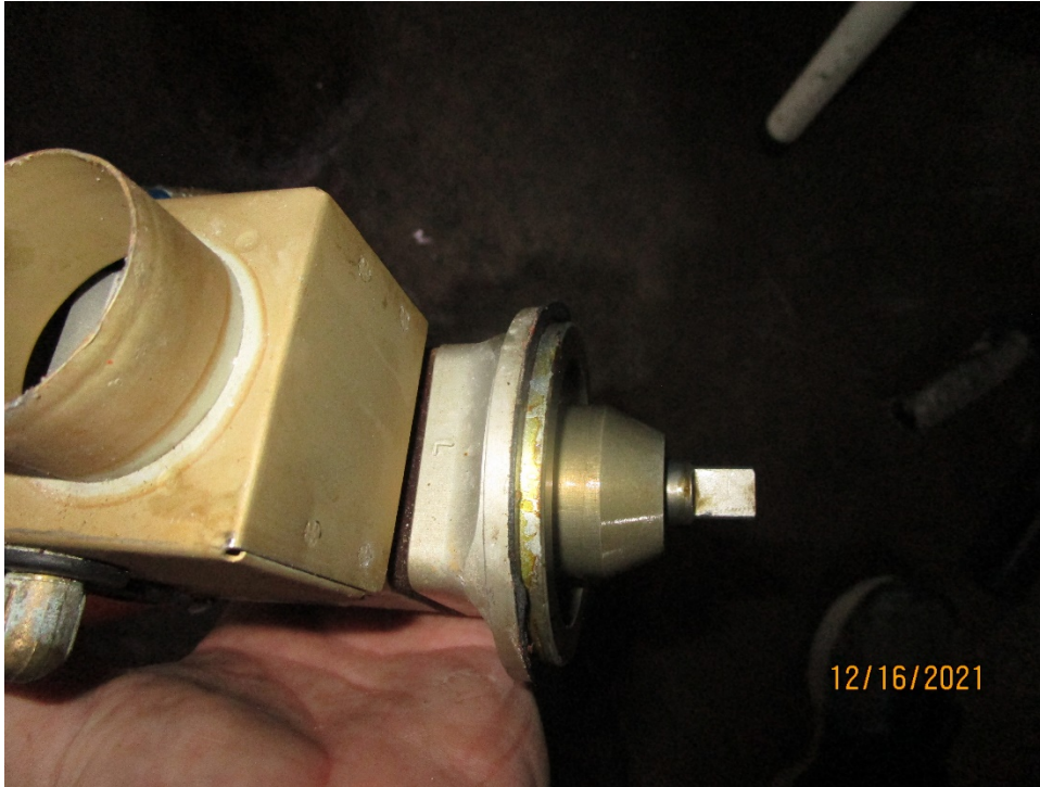
Fuel pump – drive spline intact
