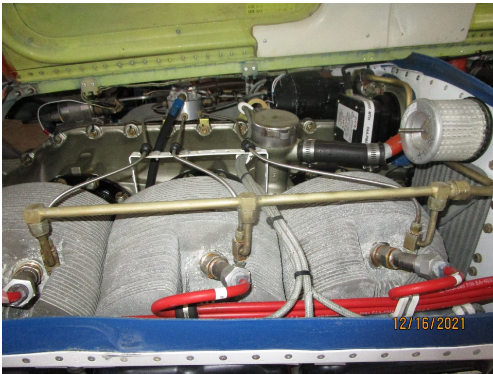
Right magneto and left electronic ignition
