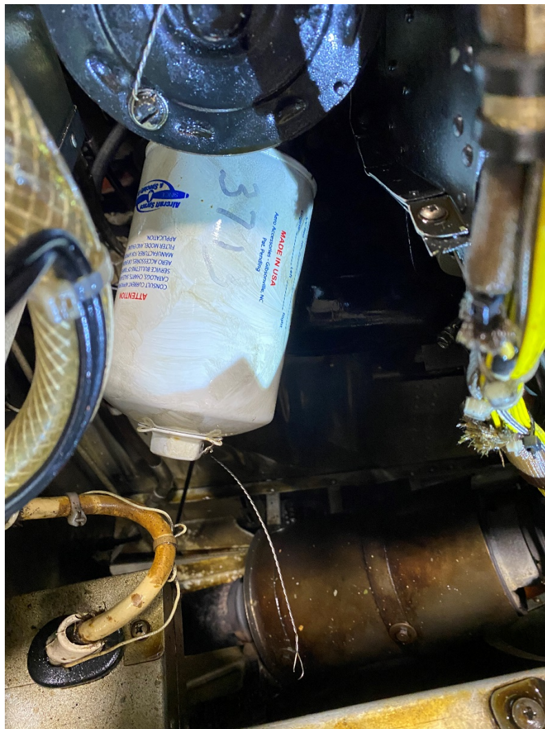
Figure 5: Fracture Separated Safety Wire
