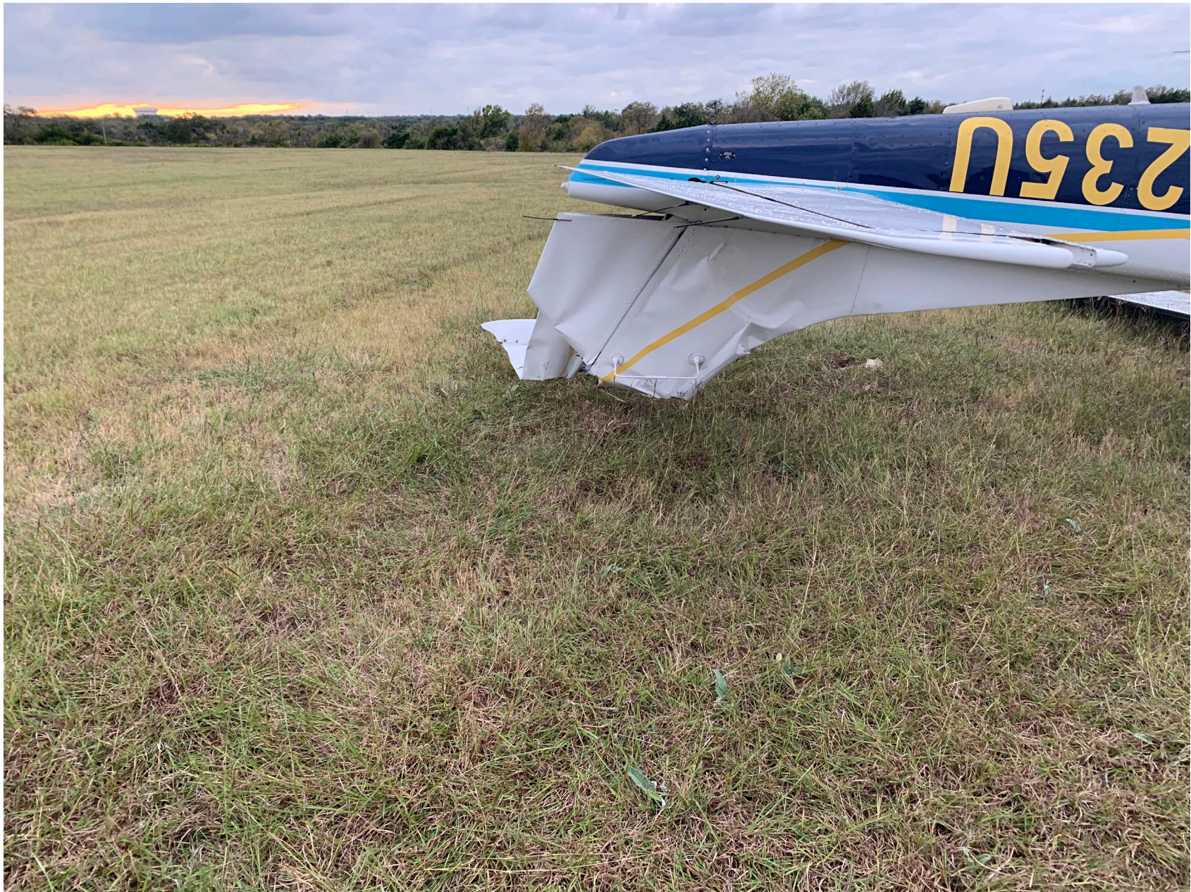
Photo 5 – View of the substantial damage sustained to the empennage (courtesy of the Federal Aviation Administration).
