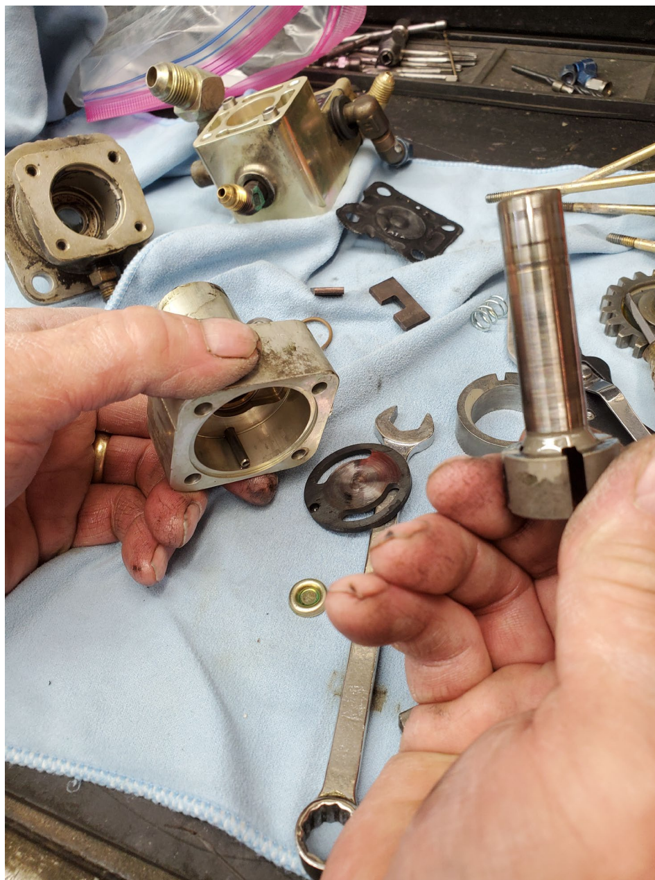
Photo 10 – View of the fuel pump being disassembled (courtesy of Aircraft Accessories of Oklahoma).
