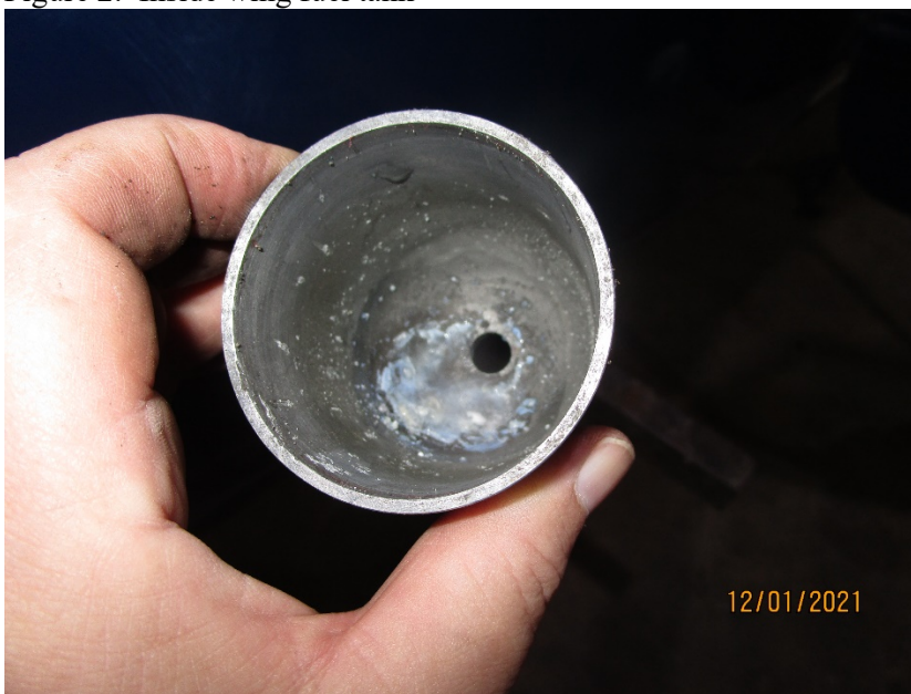
Figure 3: Unidentified contaminates in gascolator
