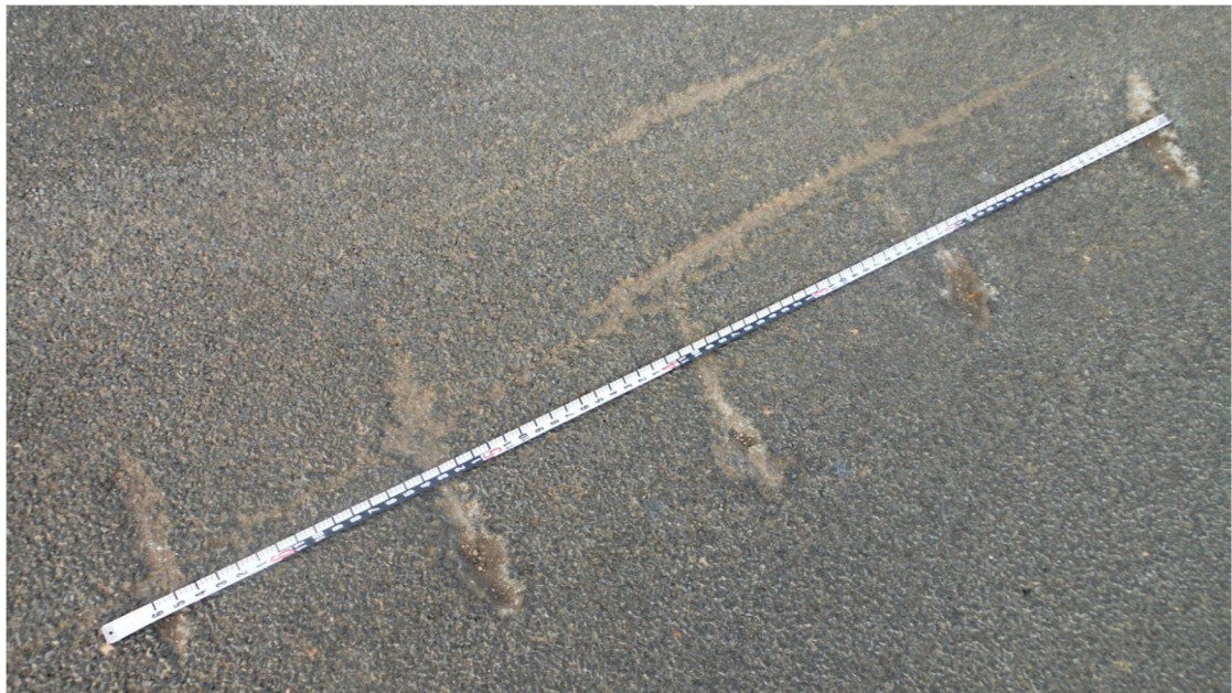
Photo 2 – Propeller Strike Marks on Road at Accident Site (Courtesy of Hartzell)
