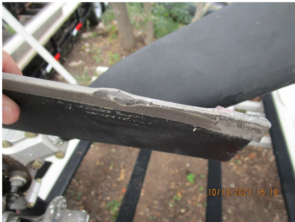
Figure 10: One blade was Bent about 7 Inches from the Hub
