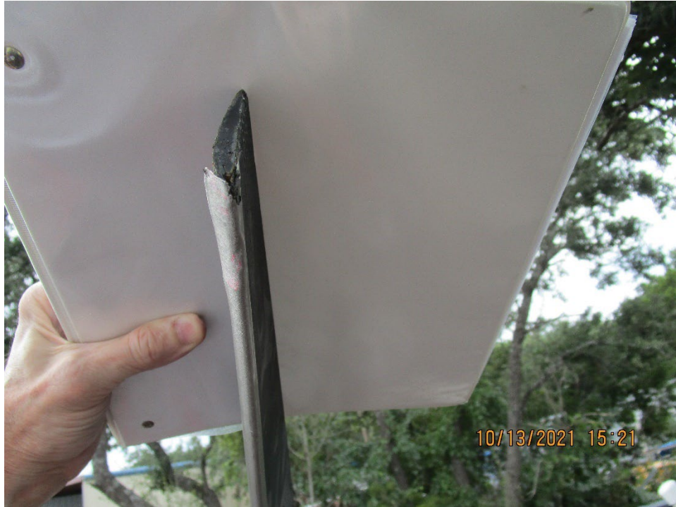
Figure 11: The Tip of the Second Blade was Fracture Separated.
