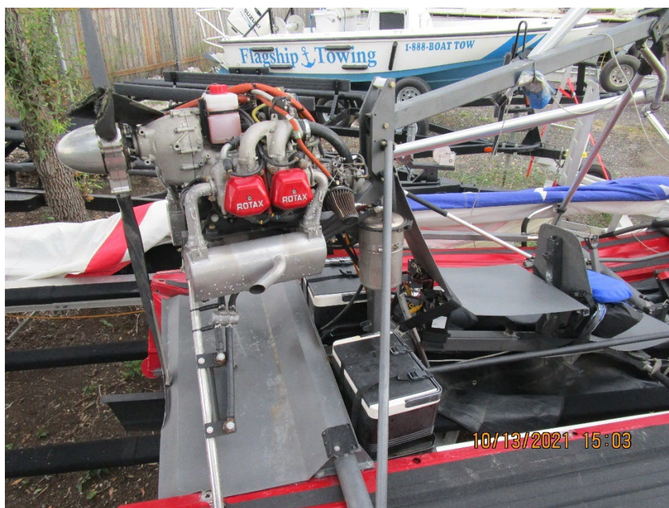
Figure 8: The Side of the Engine and Carriage Mast Bend
