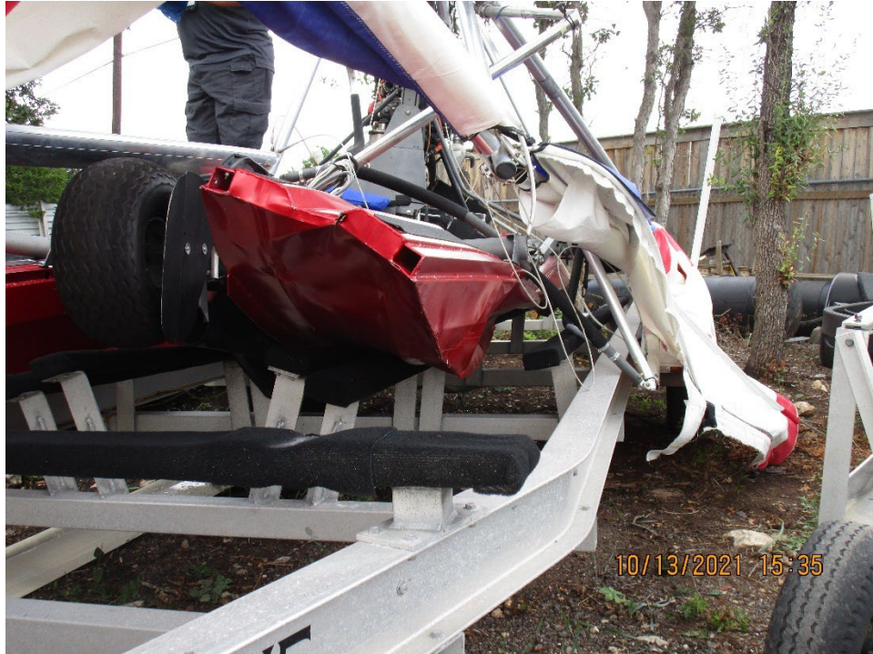
Figure 3: Left side float and left side control corner bracket.
