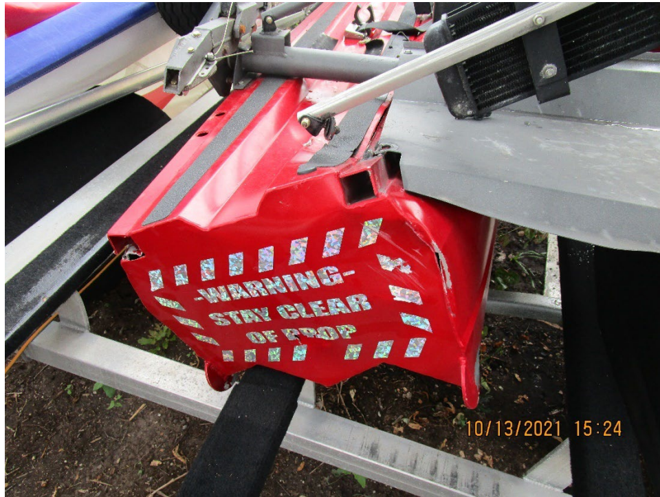
Figure 13: Score Marks on the Aft Left Float
