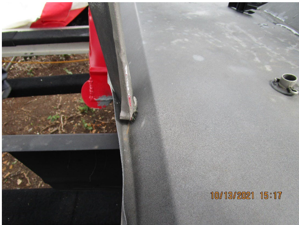
Figure 12: The Blade Tip of the Third Blade was Wedged on the Metal Plate Below the Engine
