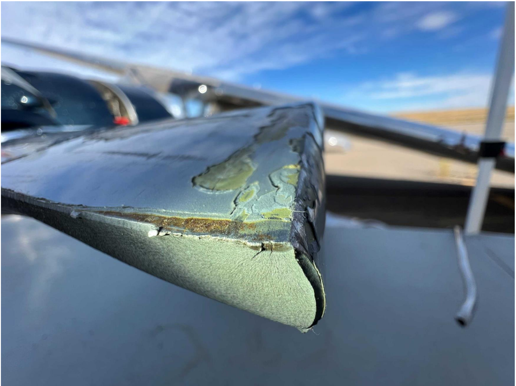
Photo 3 – Left Main Landing Gear Spring Fracture (FAA Photo)
