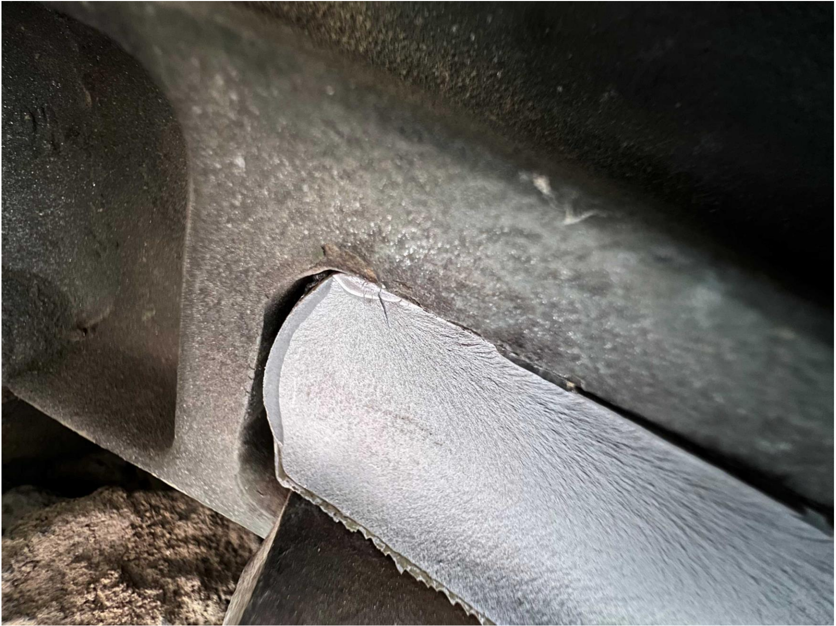
Photo 4 – Left Main Landing Gear Spring Fracture (FAA Photo)
