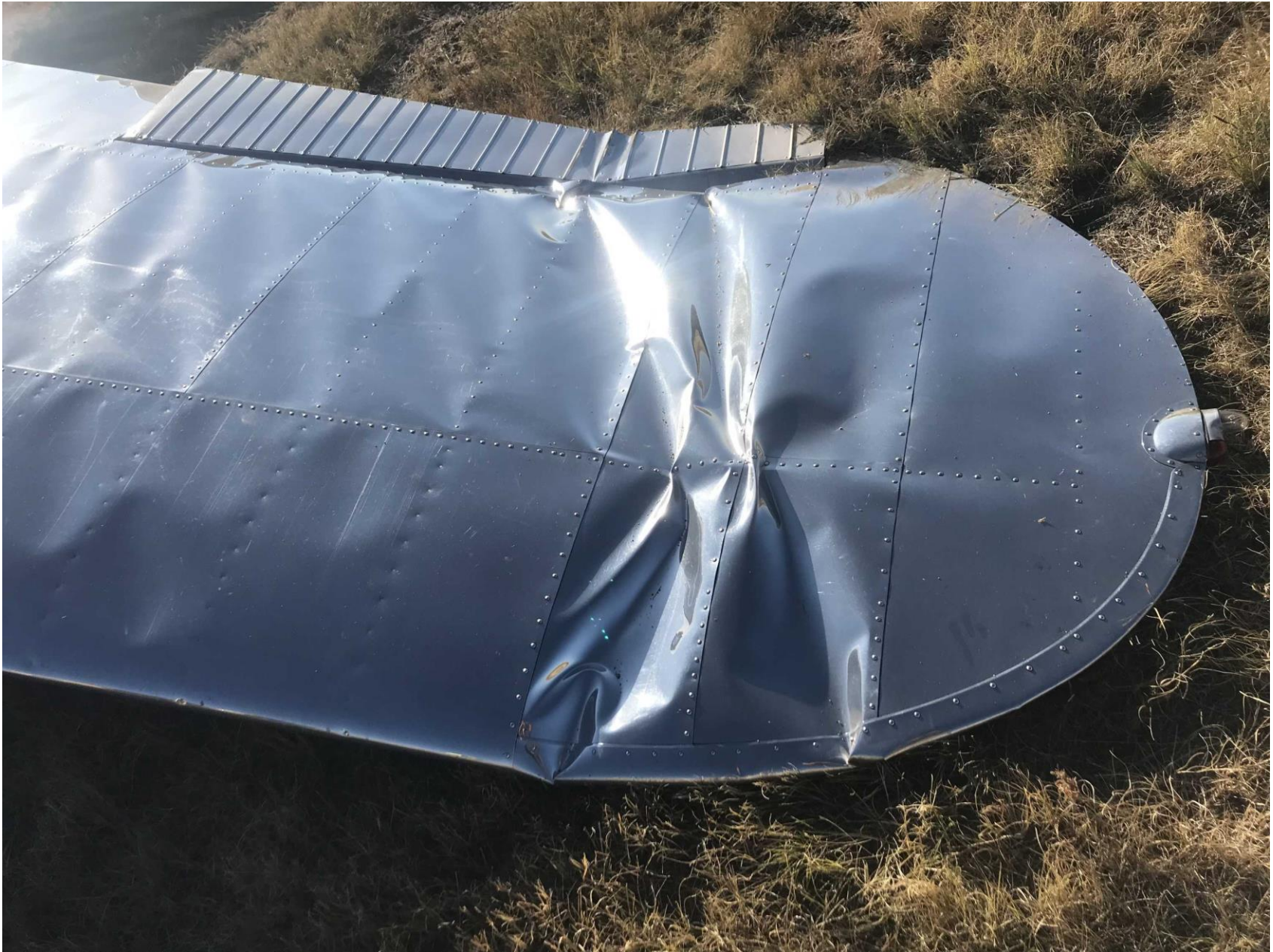
Photo 2 – Left Wing Damage (Airport Operations Photo)
