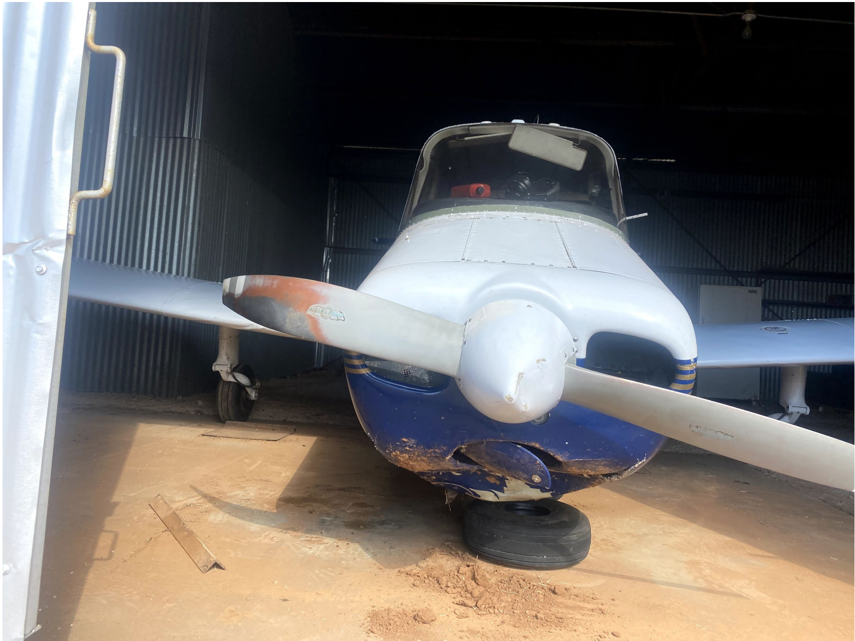
Photo 3 – Front view of airplane after recovery. Right leading edge wrinkled indicating internal damage to wing structure. (Photo provided by pilot)
