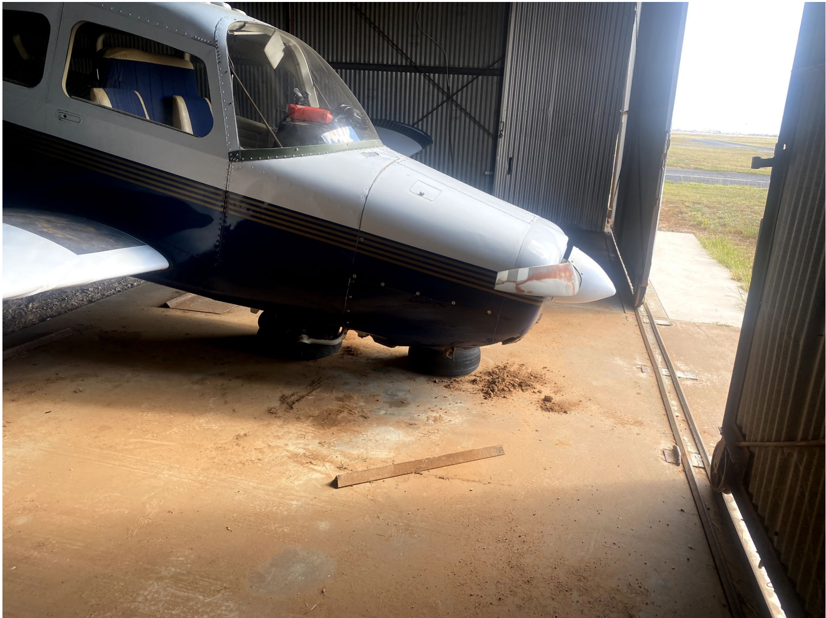
Photo 2 – Right side view of airplane after recovery. Right wing leading edge wrinkled indicating internal damage to wing structure. Forward fuselage side wrinkled indicating substructure damage. (Photo provided by pilot)
