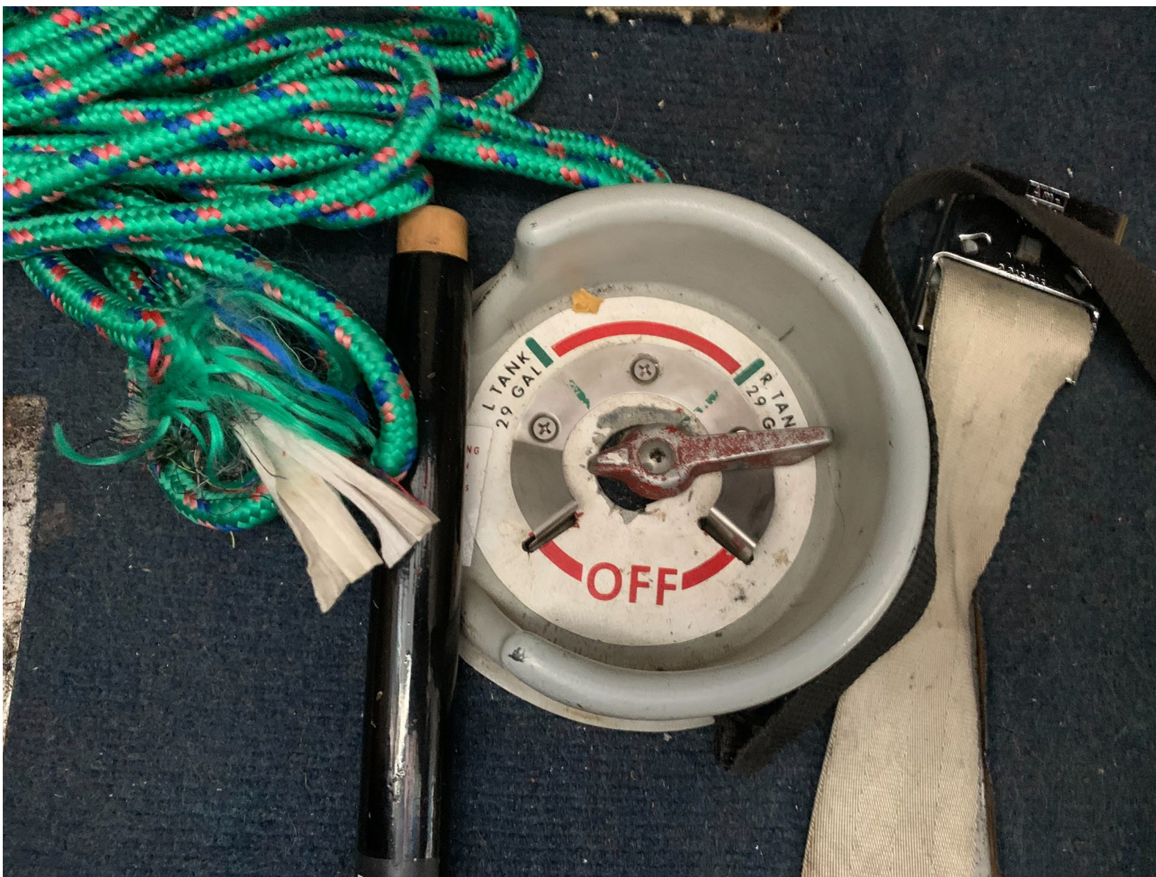
Photo 4 – Fuel selector valve as found after the accident (FAA Photo)
