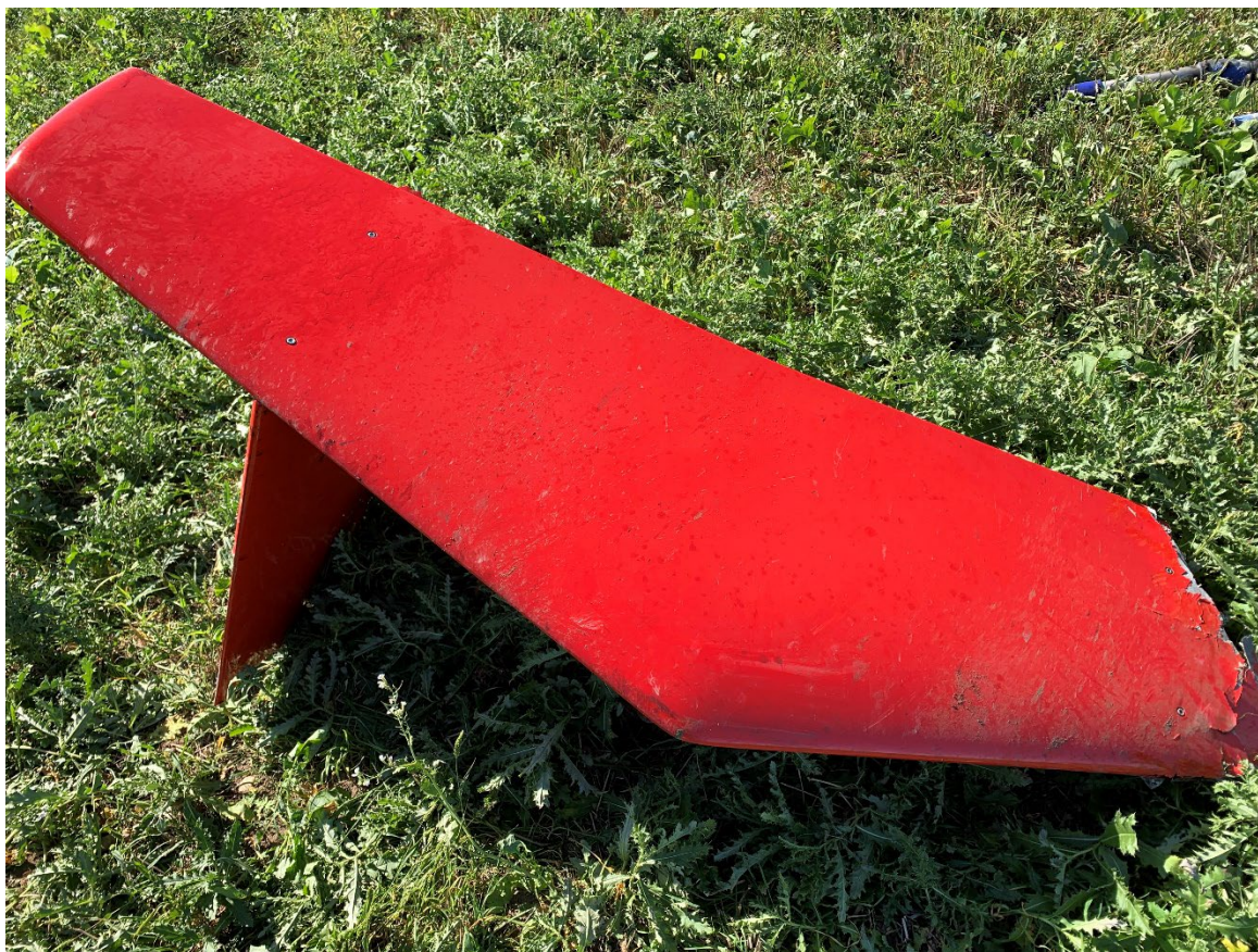
Photograph 6 - View of the empennage with fluid spray at the accident site.
