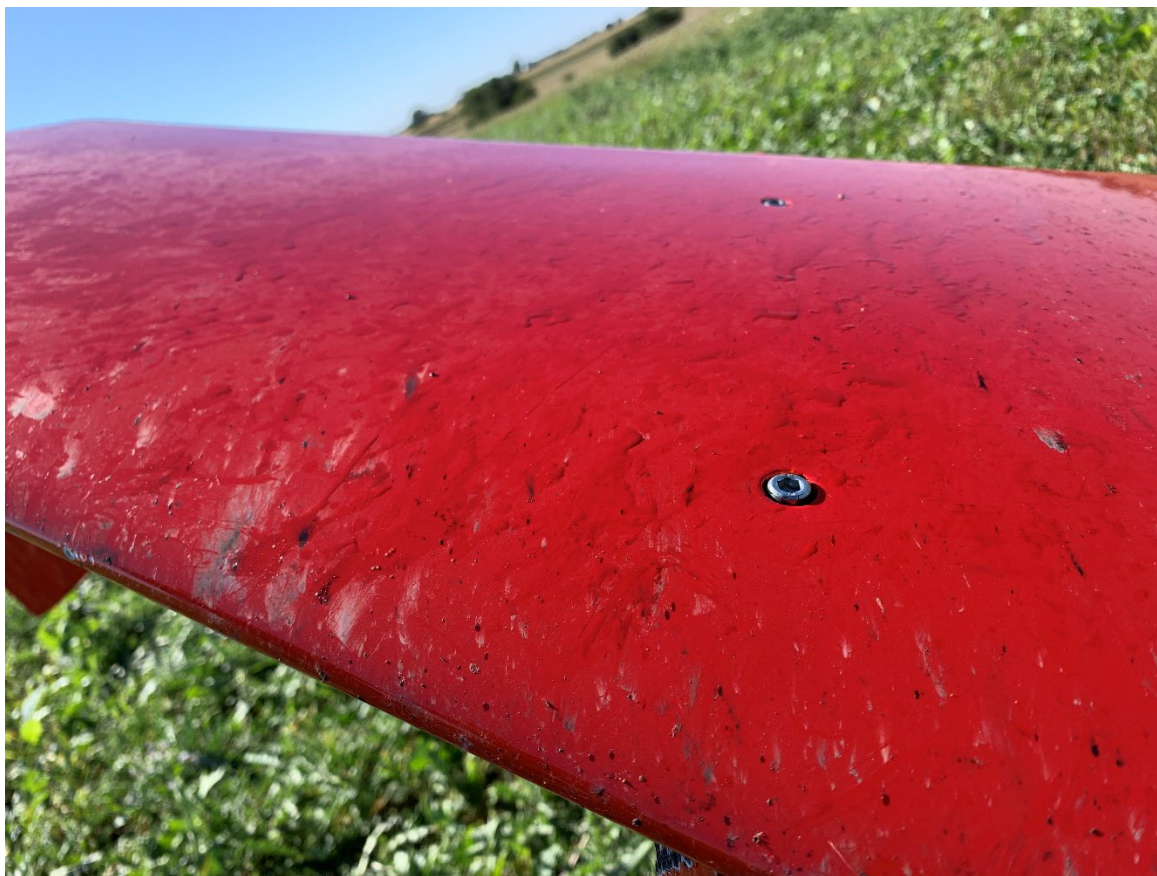
Photograph 7 - View of the empennage with fluid spray at the accident site.
