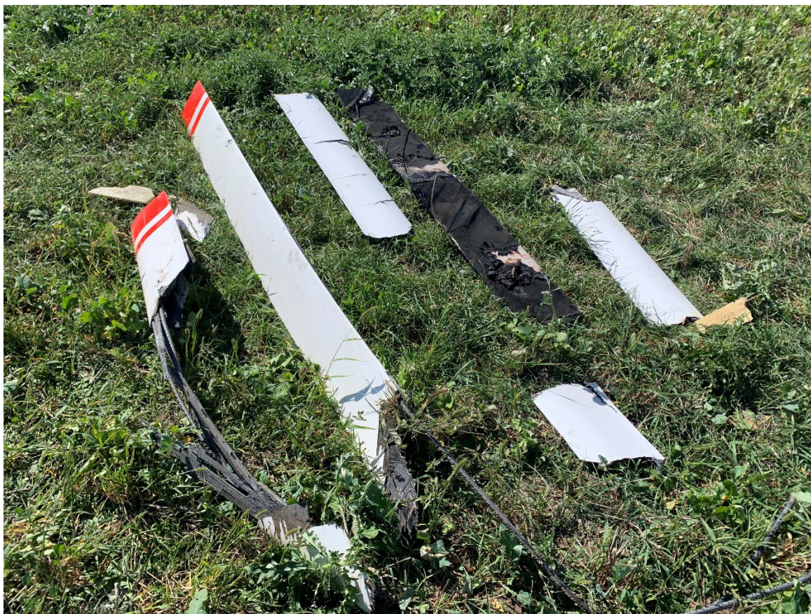
Photograph 5 - View of the main rotor blades at the accident site.
