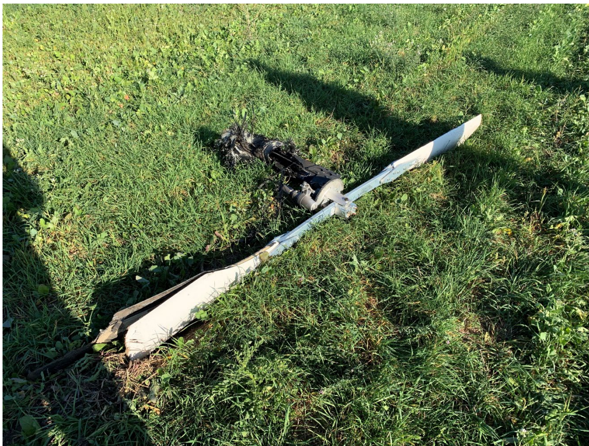
Photograph 4 - View of the main rotor mast at the accident site.
