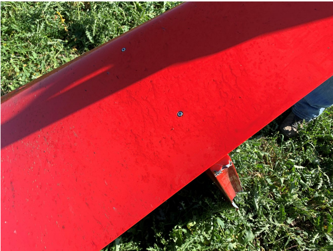
Figure 6. Fluid on exterior surface of aircraft
