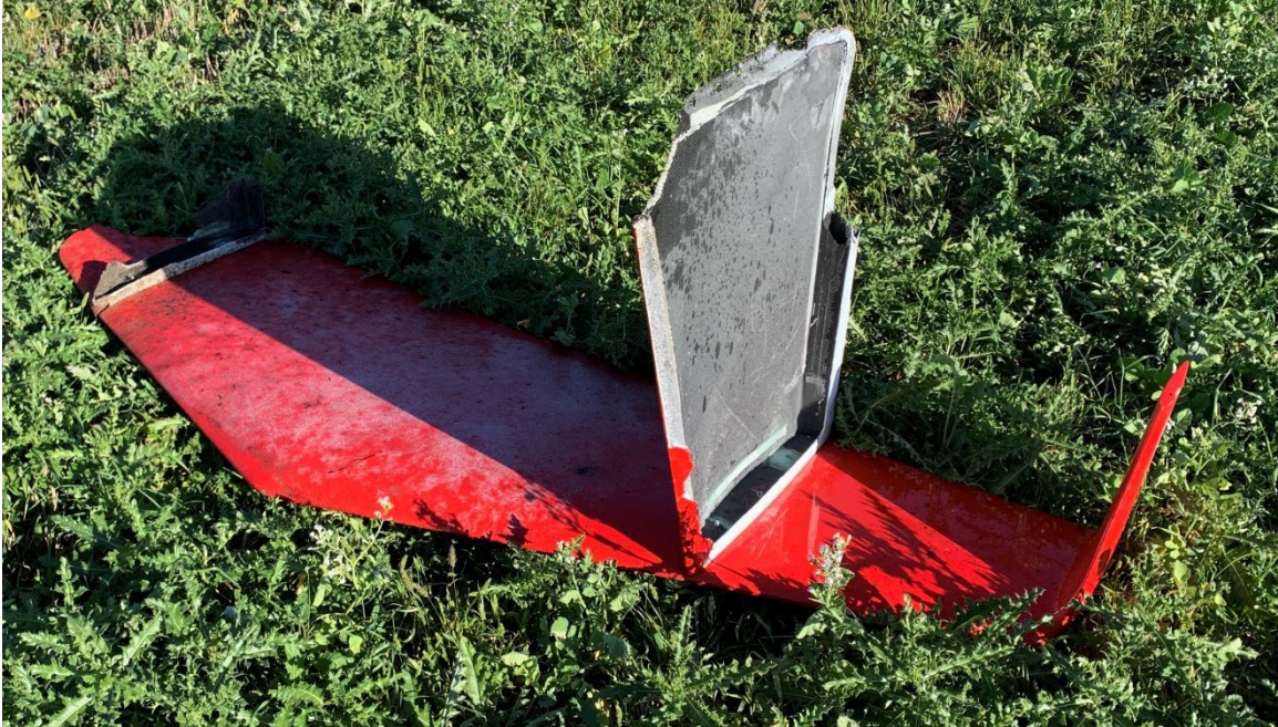
Figure 7. Fluid spray on interior of empennage.
