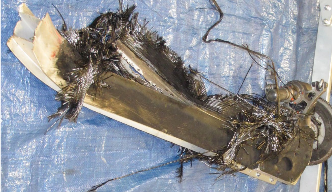
Figure 9. Close up photograph of thermal damage to rotor mast.
