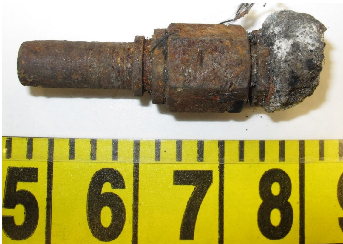
Figure 16. Separated frange connector.
