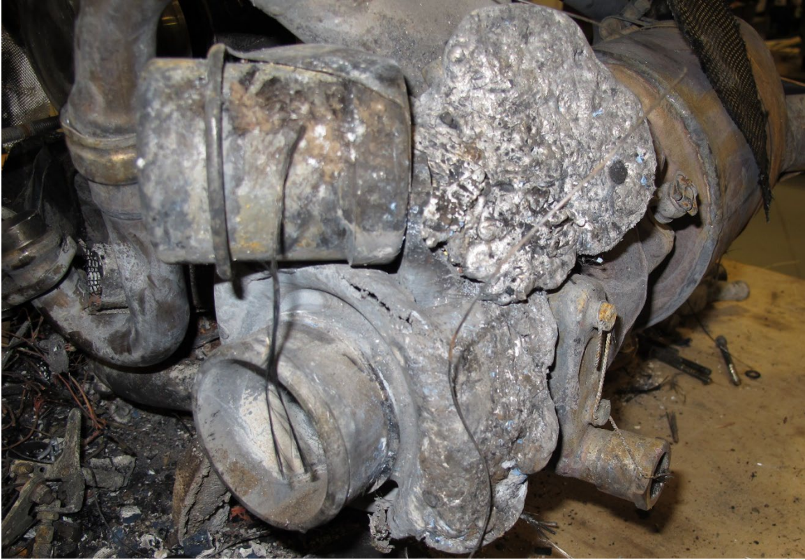
Figure 18. Turbocharger intake ("cold" side).
