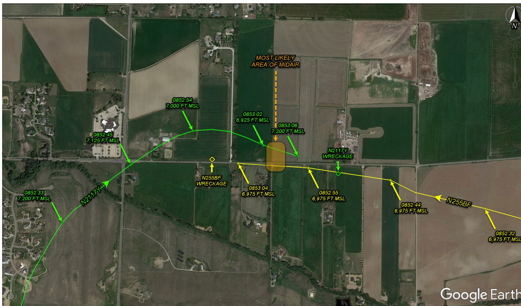
Figure 1. Sonex and Cessna Airplanes' Flight Tracks.
