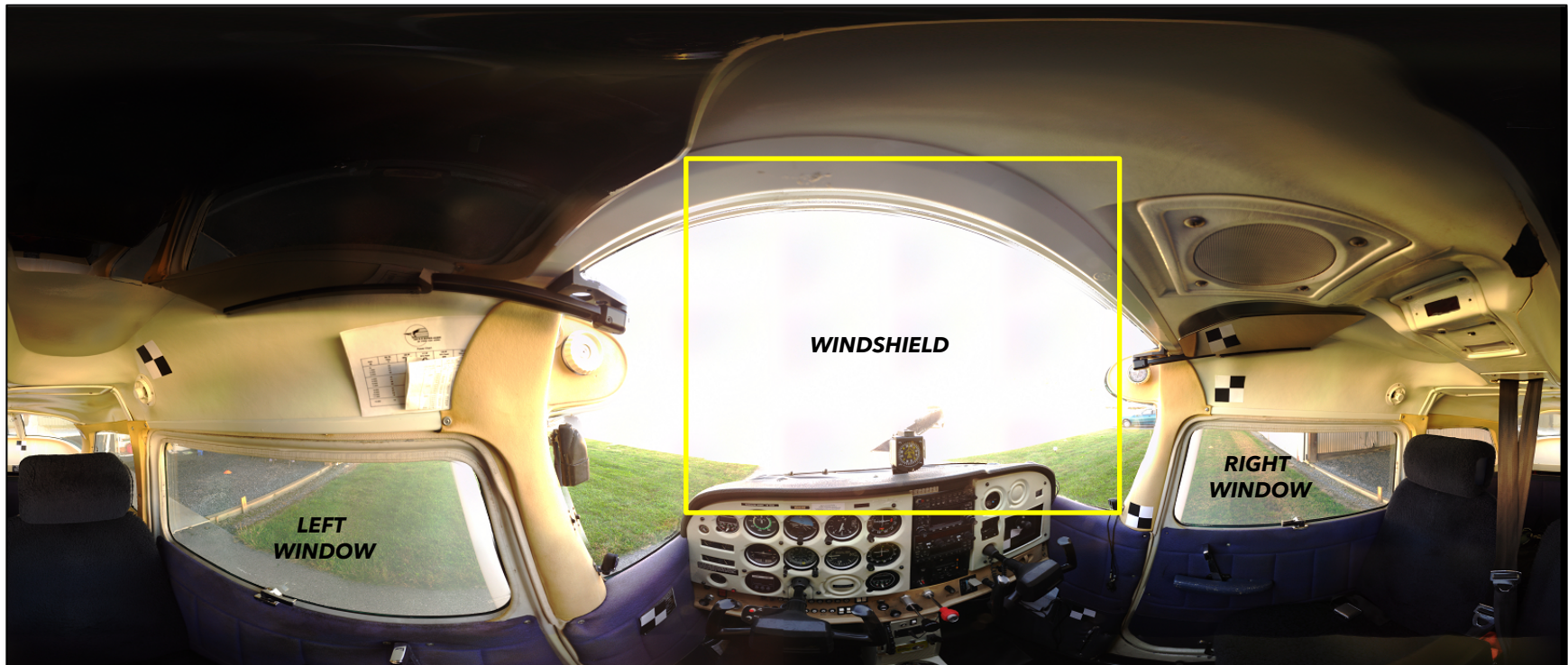
Figure 16a. Color image of the 360° laser scan from the left seat of the exemplar Cessna172. The yellow box highlights the area depicted in Figure 14a.
