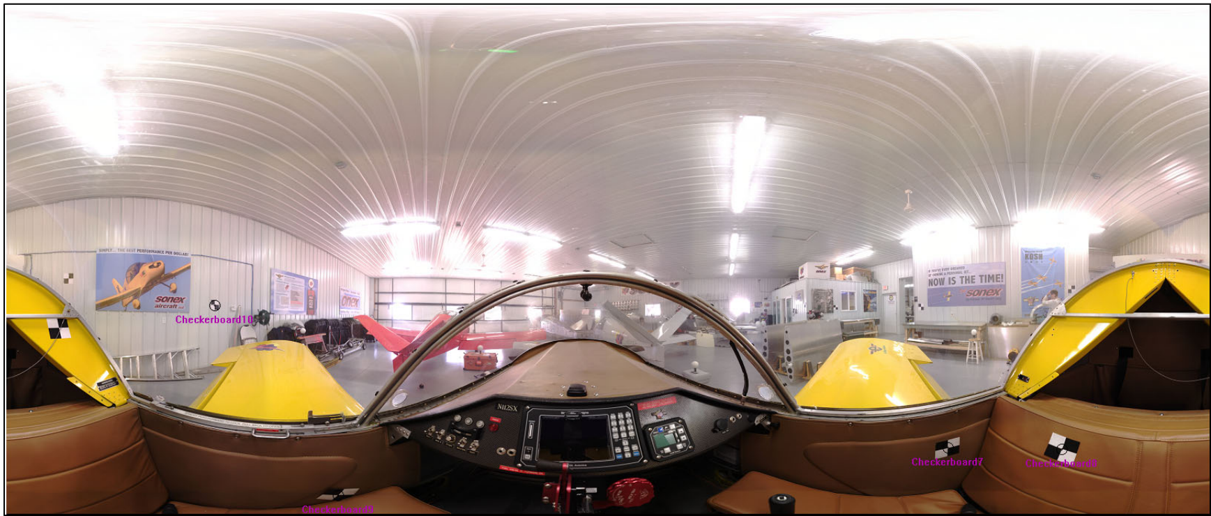
Figure 17b. Color image of the 360° laser scan from the right seat of the exemplar Sonex, with the cardboard template removed, depicting the original exemplar airplane configuration.
