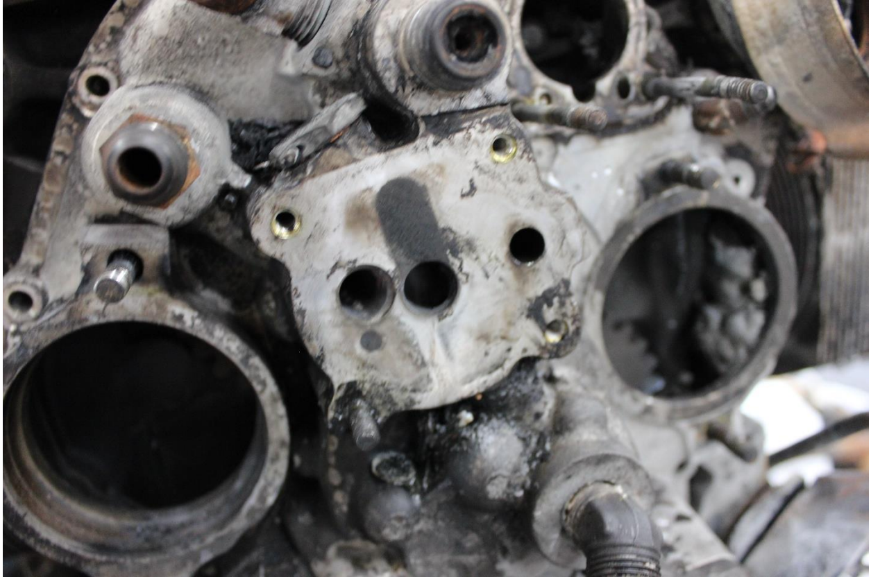
Photo 2: Vacuum Pump Drive Pad (NTSB Photo)
