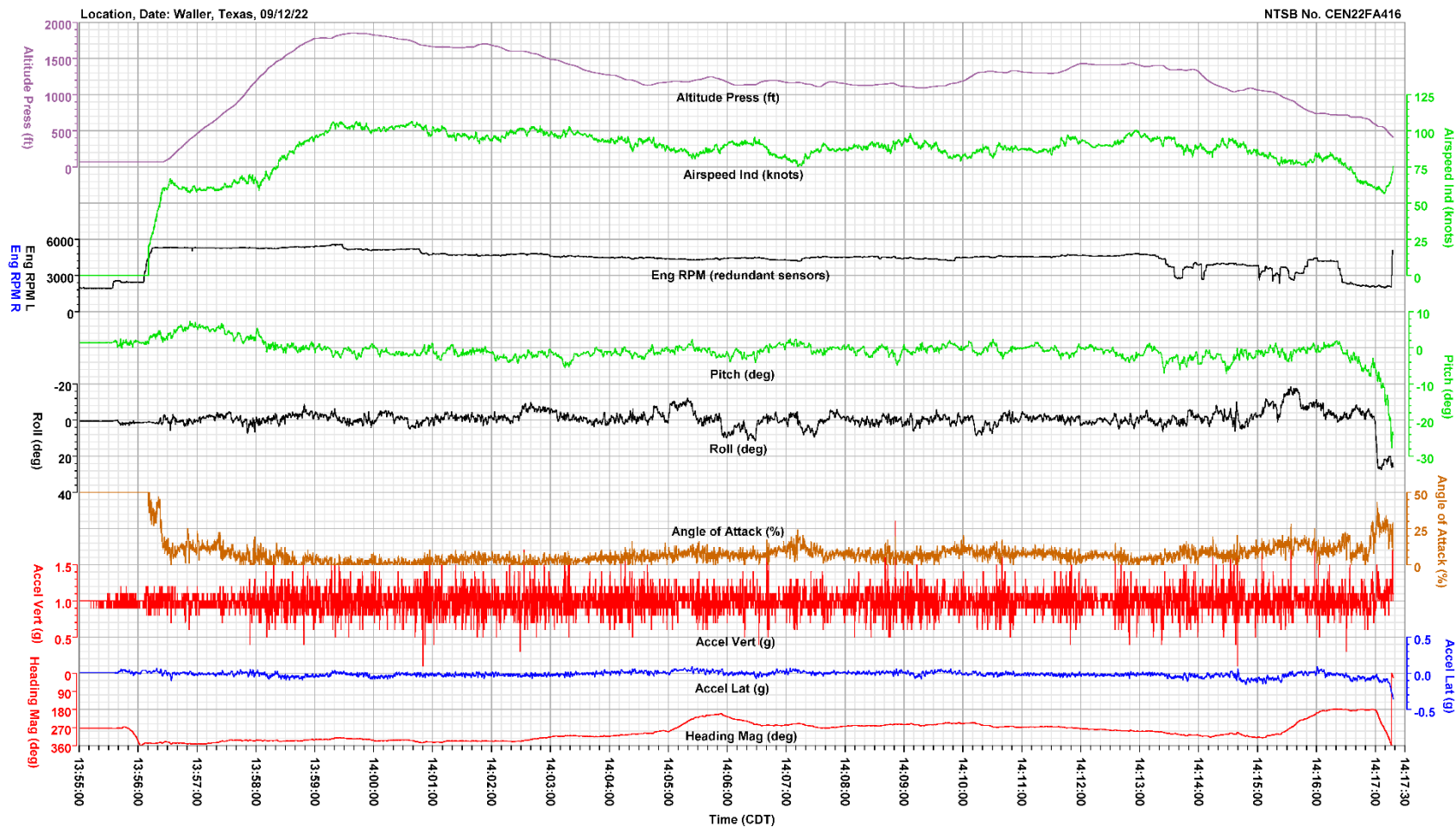
Figure 5. Plot of recorded aircraft basic parameters from accident flight.
