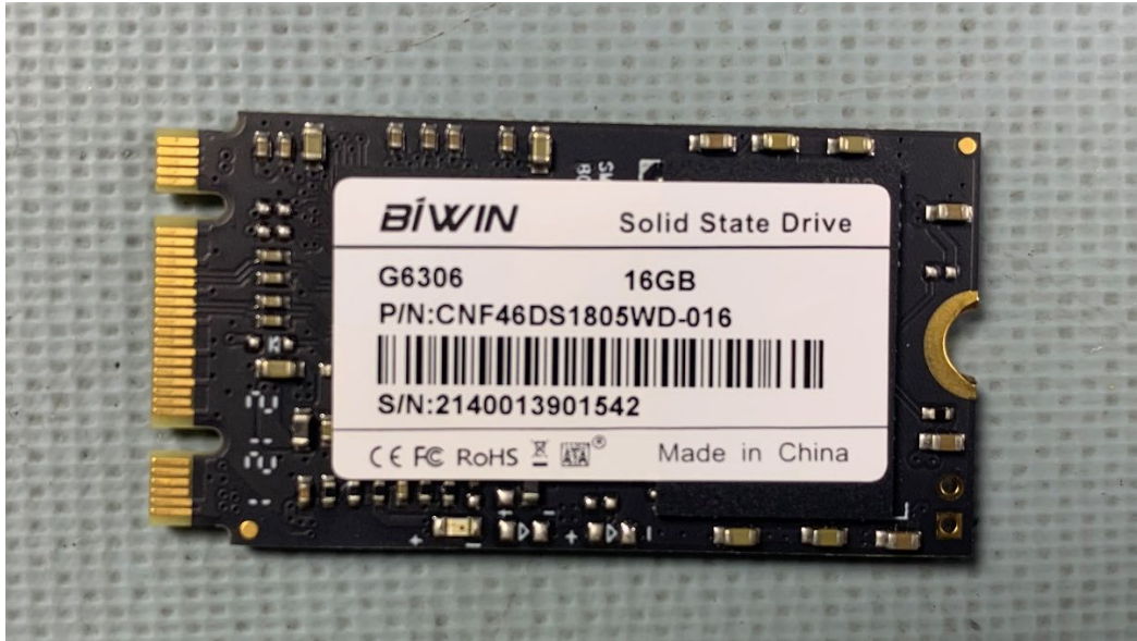
Figure 2. Memory module (DOM) removed from the recorder.
