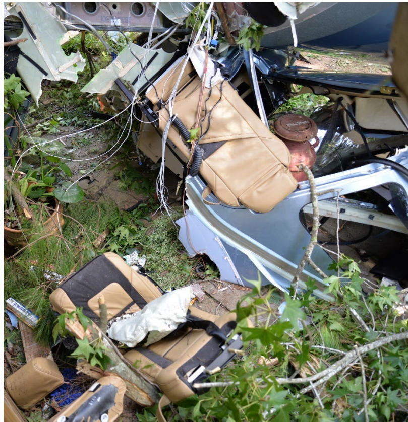
Figure 3. Front seats as found at the accident site.
