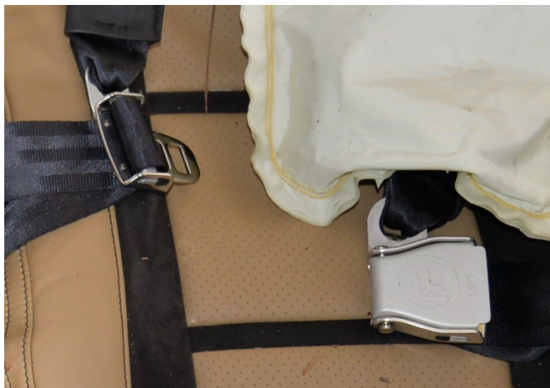
Figure 14. Seat 2 showing plugs in the correct position.
