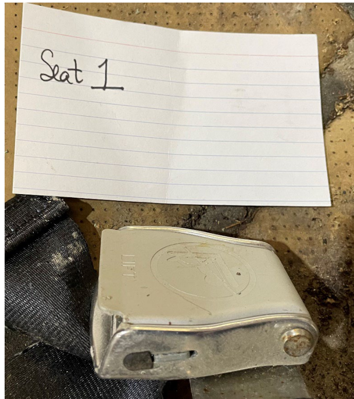
Figure 11. Seat 1's buckle with anti-rattle plug in the incorrect position.
