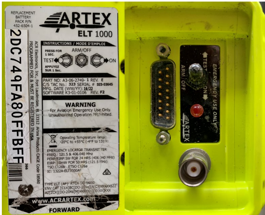
Figure 17. ELT information, including the ARM/OFF switch position.
