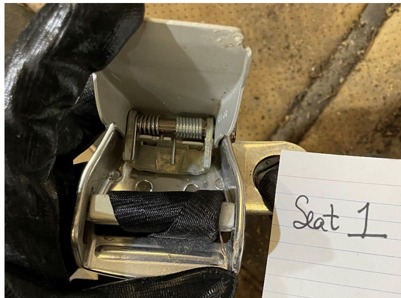
Figure 12. Seat 1's buckle with webbing twisted around the webbing load bar.
