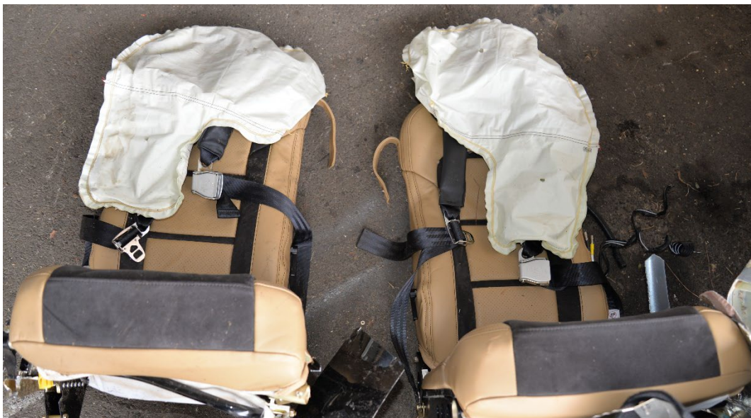
Figure 9. Front crew seats with deployed airbags.
