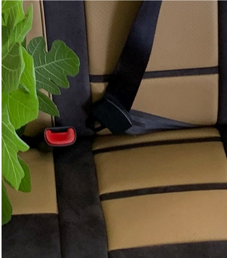
Figure 16. The push button buckle for the rear seat positions.
