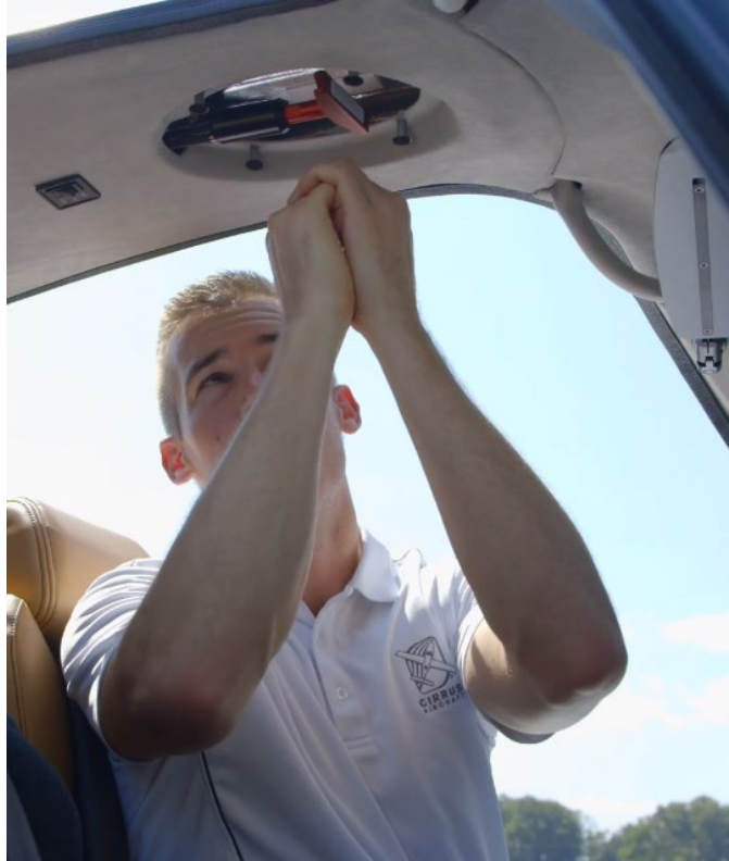
Figure 18. Cirrus employee demonstrating the location and how to operate the CAPS handle. (Source: Cirrus website)
