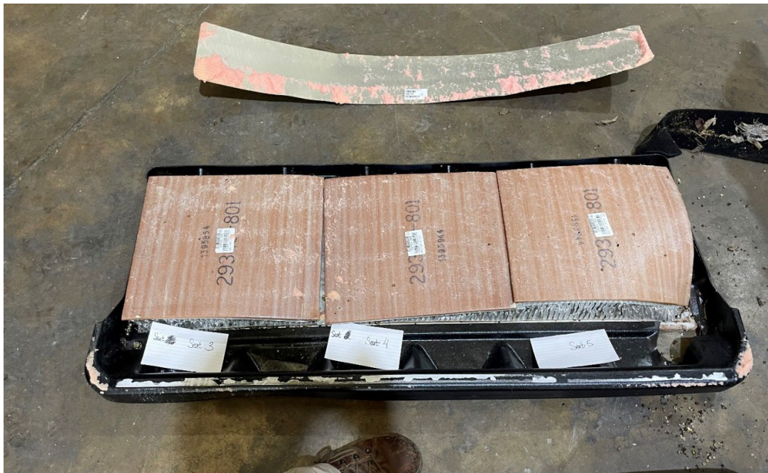
Figure 8. Rear seat with leather cover and foam removed.
