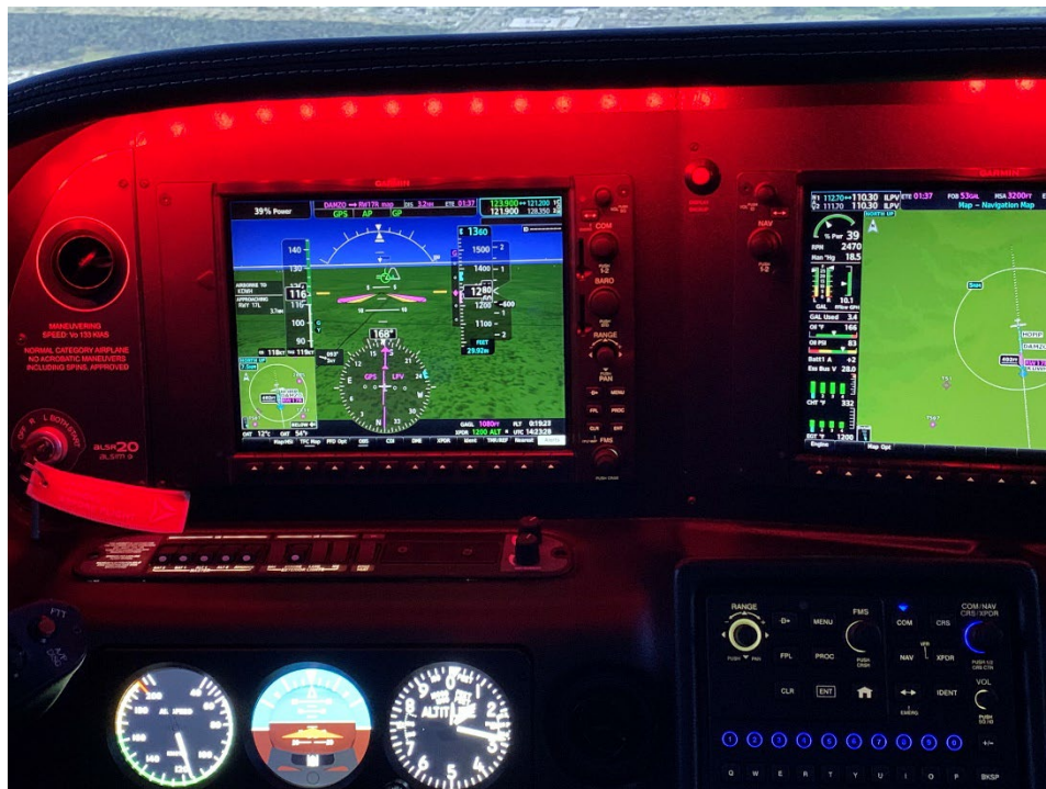
Figure 2: SR20 Simulator PFD and MFD
