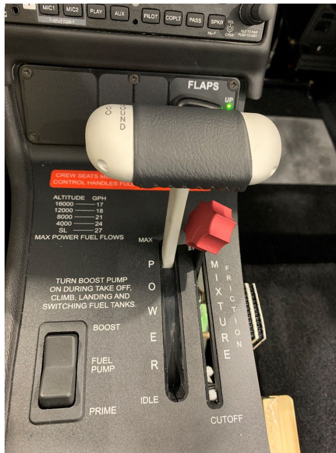
Figure 3: Throttle quadrant and fuel mixture control lever
