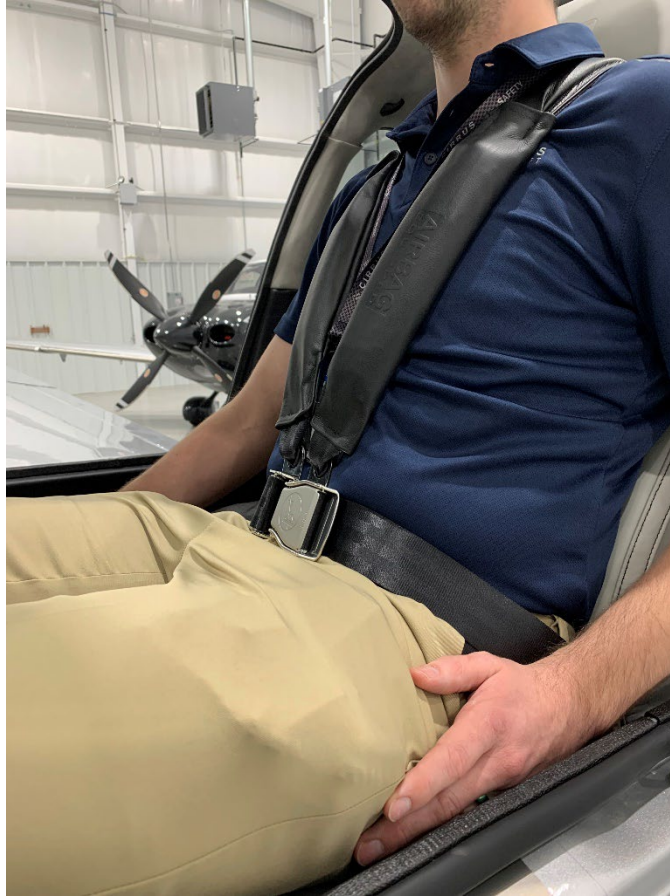
Figure 4: Photo documentation of 4-point seat restraint.
