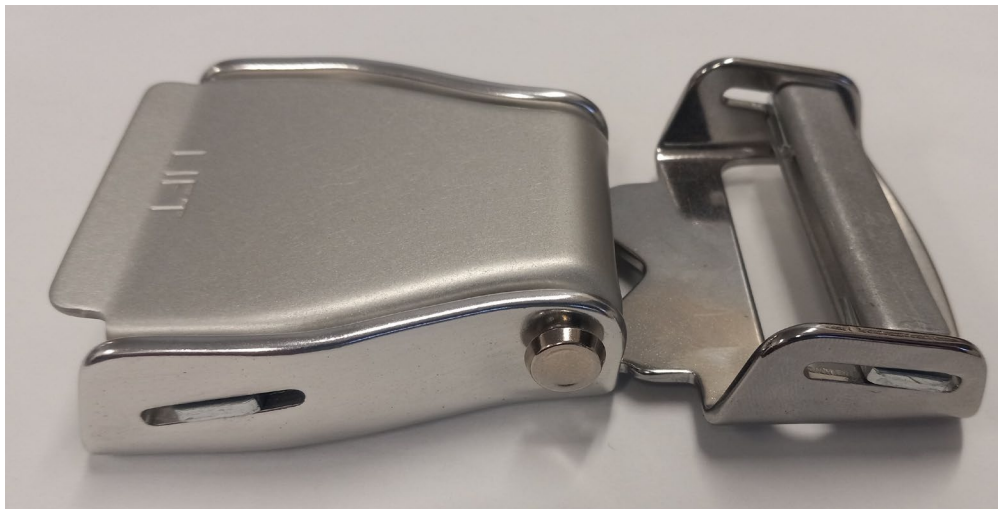
Figure 3. Buckle/Connector Before Plug Installation
