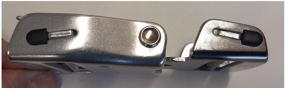
Figure 2. Buckle/Connector with Incorrect Plug Installation
