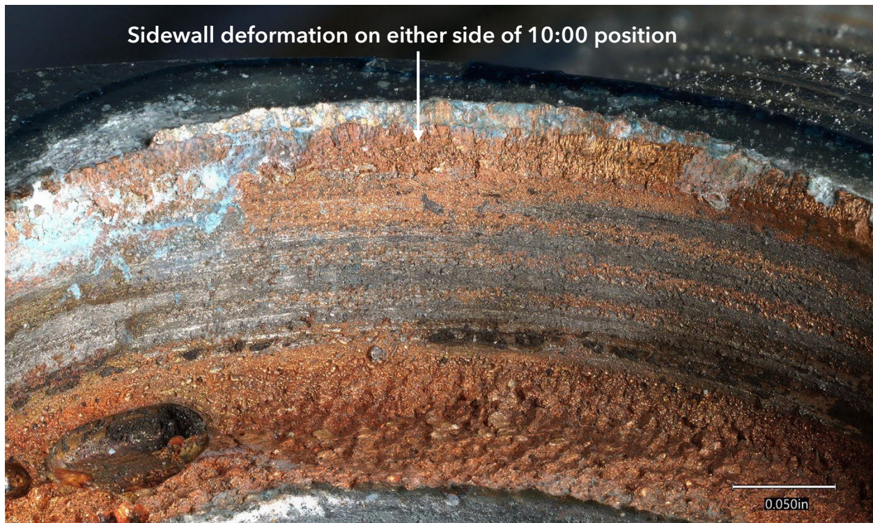
Figure 7. Image of the socket sidewall centered about the 10:00 position with an indicator pointing to deformation of the sidewall edge at the entrance to the joint.
