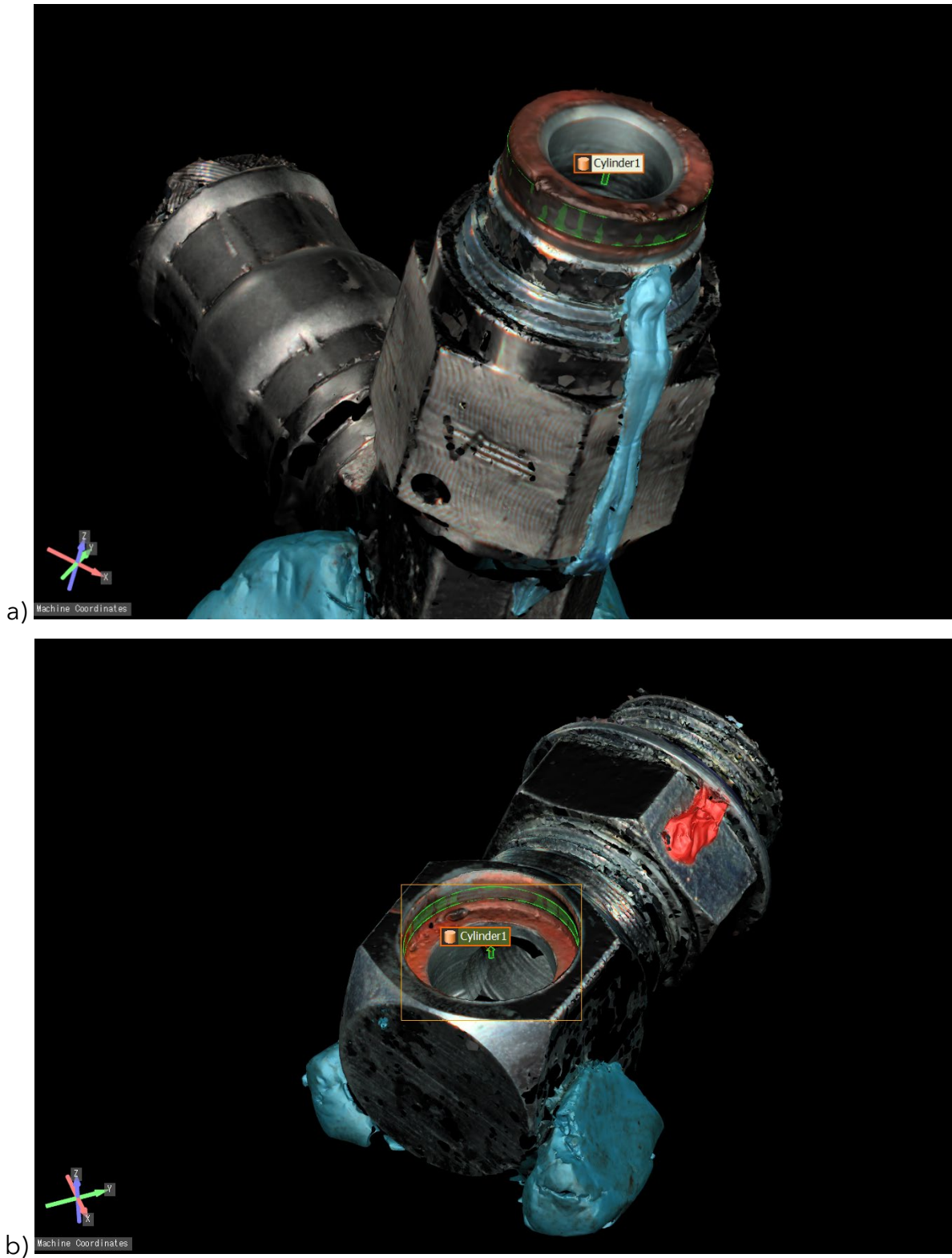
Figure 9. 3D models generated using a structured-light 3D scanner; a) tube-side of joint and b) socket-side of joint.
