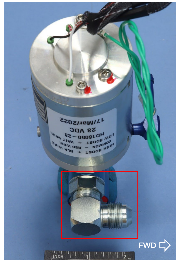
Figure 2. Two images showing different views of an exemplar fuel boost pump with red rectangles highlighting the 90° elbow fitting. The pump is installed on the right side of the aircraft. The left image shows the forward-facing side of the pump and the right image shows the right and top sides of the pump.
