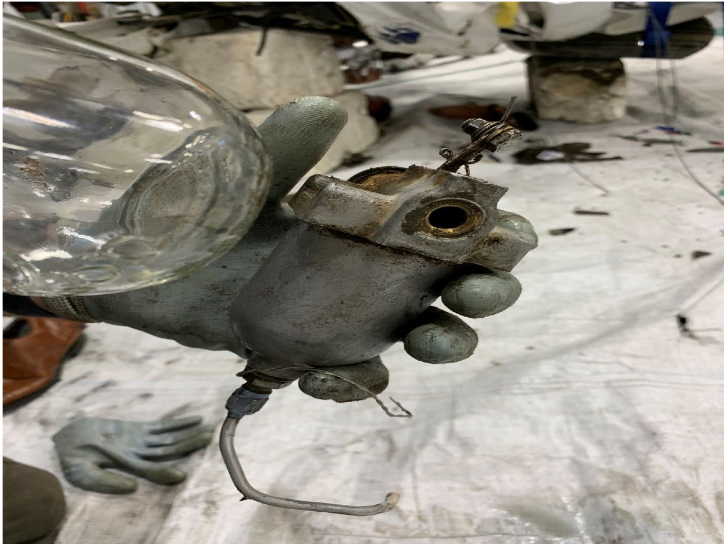
Photograph 6 - Gascolator Contents (NTSB)
