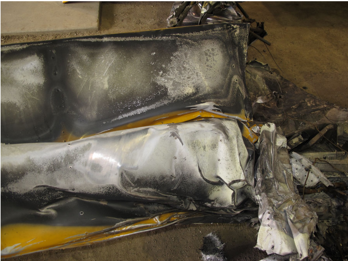
Figure 2. Closeup of thermal damage to left wing.
