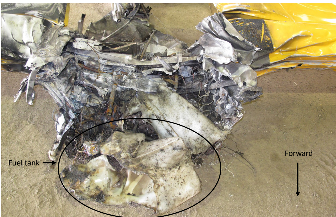
Figure 4. Closeup of aircraft cabin and fuel tank.
