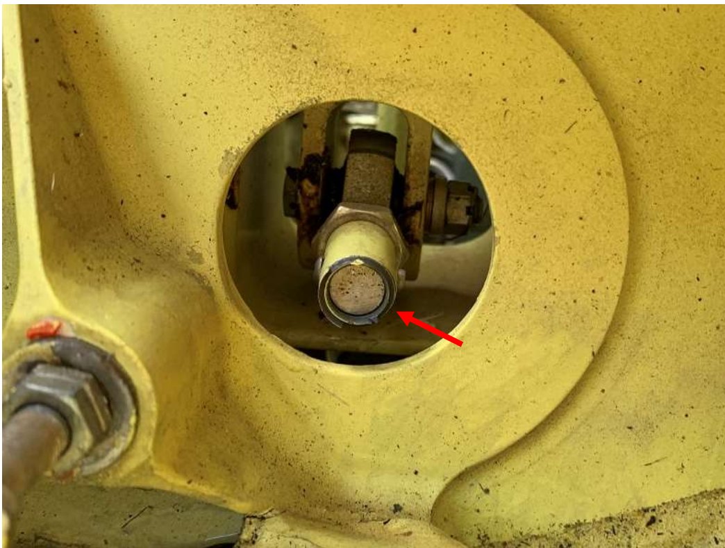
Figure 2. The red arrow points to the forward rod end of the left yaw/right roll control rod.
