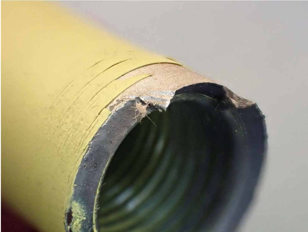
Figure 5. A closeup of the fracture surface of the left yaw/right roll control rod. (Image courtesy of Honeywell)
