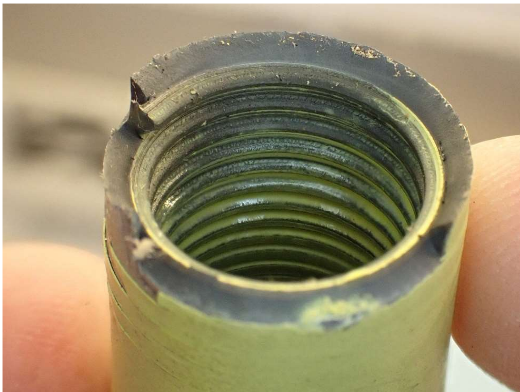
Figure 4. A closeup of the fracture surface of the left yaw/right roll control rod. (Image courtesy of Honeywell)
