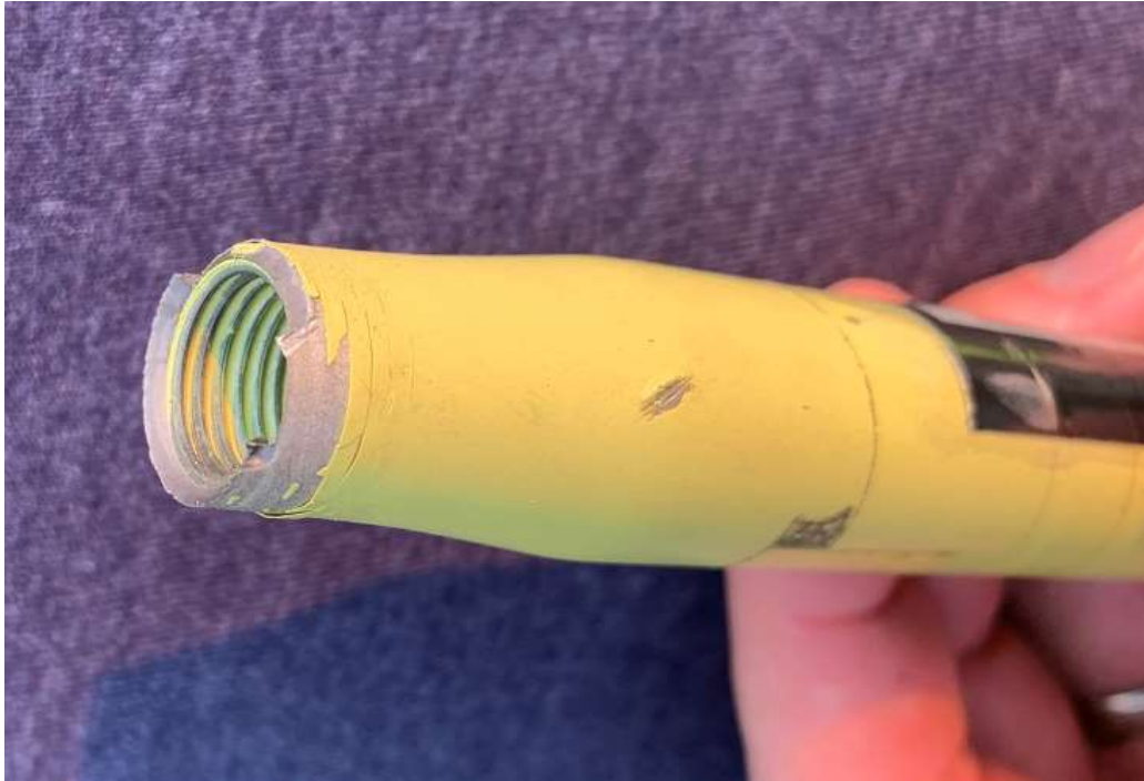
Figure 3. The fractured forward end of the left yaw/right roll control rod.
