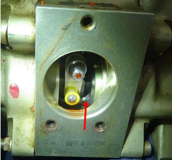
Figure 19. The crack (red arrow) as seen on the outer sleeve after removal of the cam cover.
