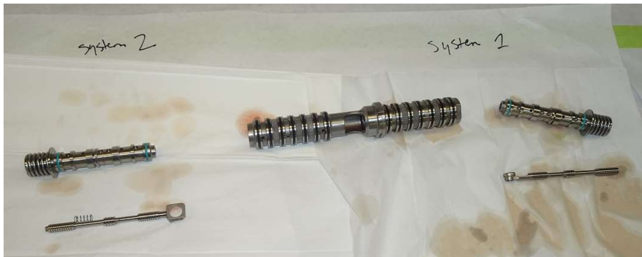
Figure 22. The spools and sleeves from the two systems of the yaw ILCA.
