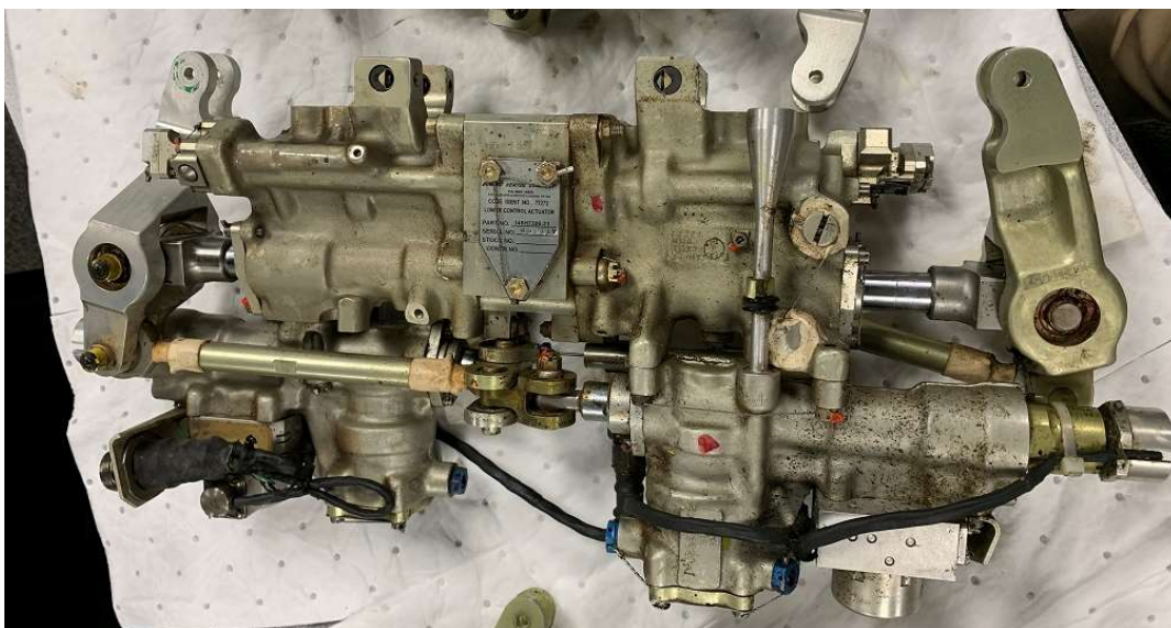
Figure 17. The yaw ILCA.
