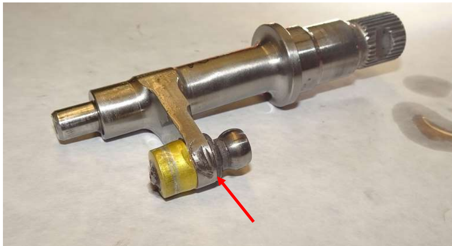
Figure 21. The red arrow points to the impact mark on the cam of the yaw ILCA.
