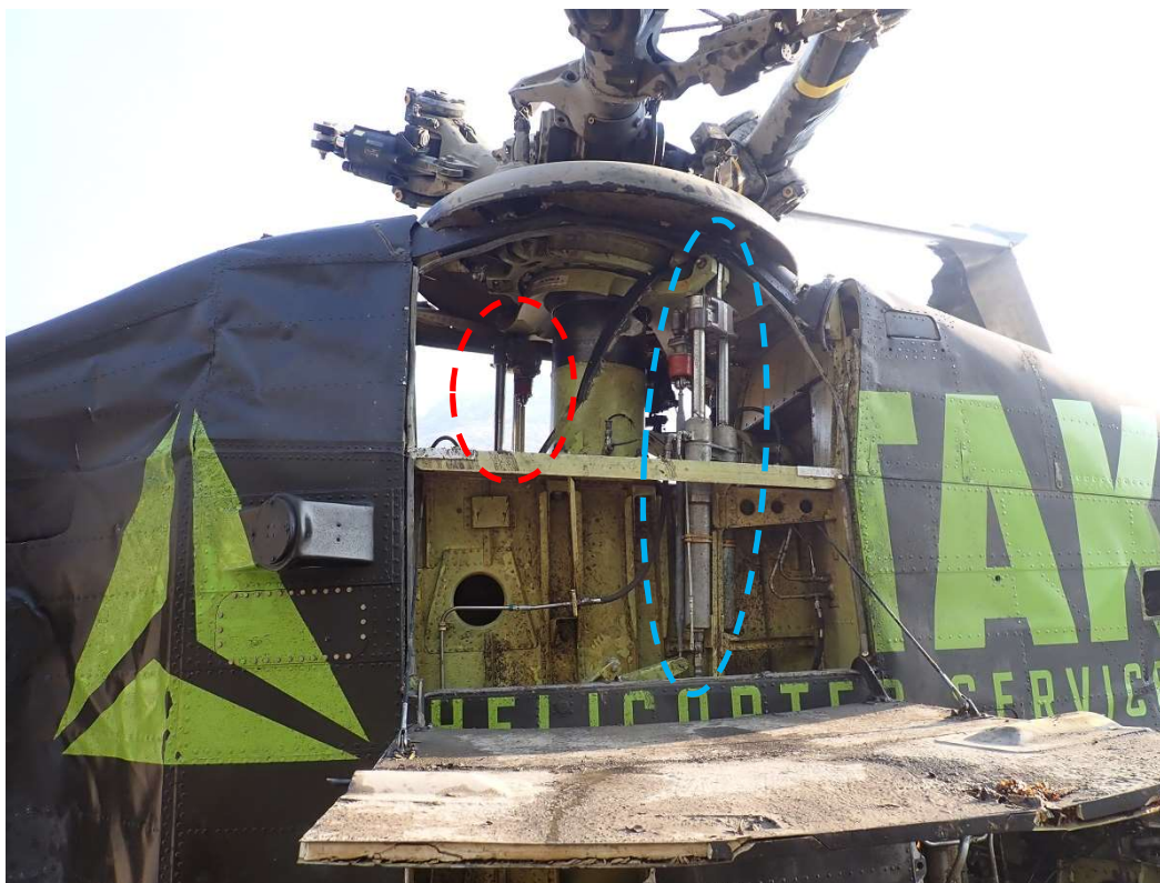
Figure 10. The aft rotor's swiveling UBA (blue dashed circle) and the upper portion of the pivoting UBA (red dashed circle). (Image courtesy of Honeywell)
