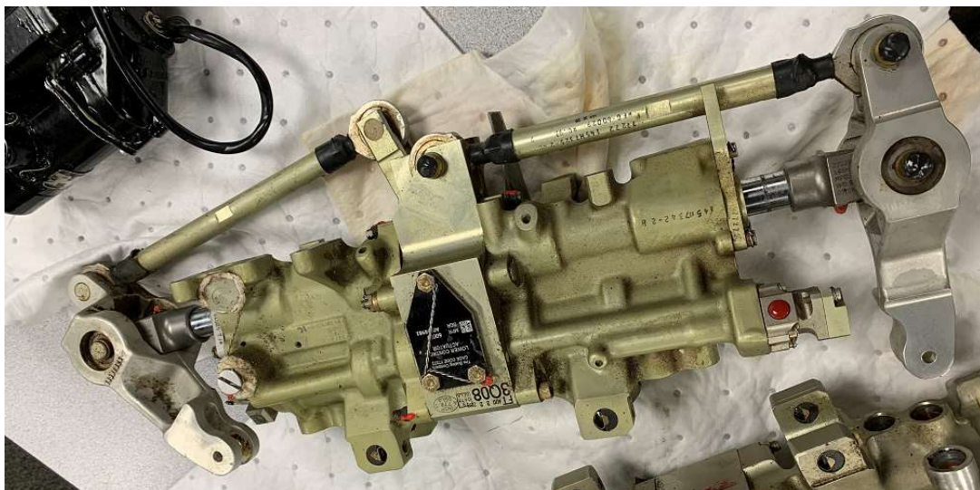
Figure 18. The thrust ILCA.
