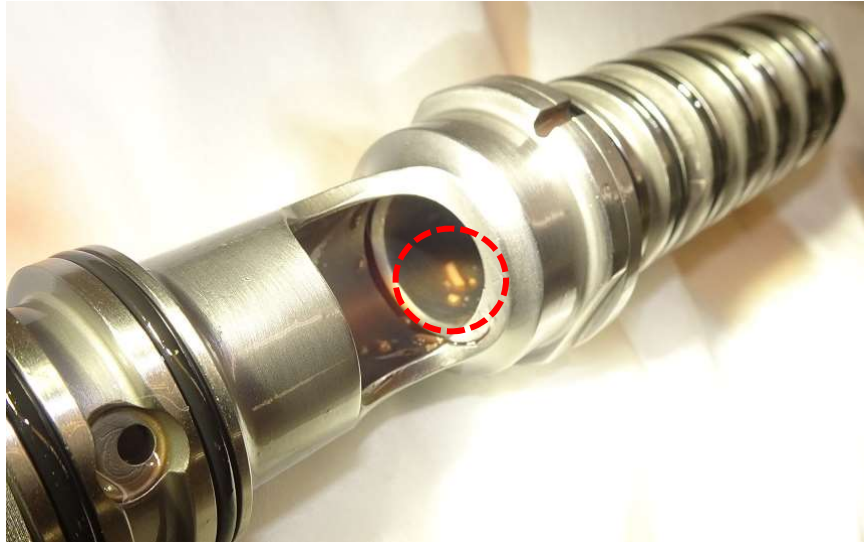
Figure 23. The white-colored material (red circle) observed within the No. 1 side of the outer sleeve of the yaw ILCA.
